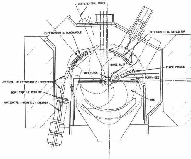
Figure 1 : View of the injector
