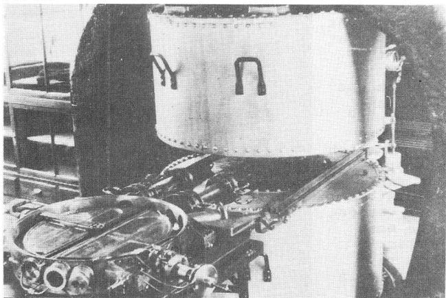
Fig.1 The first Japanese cyclotron at RIKEN, 26 inches 23 tons, obtained the first beam of 3 MeV deuterons in 1937.
