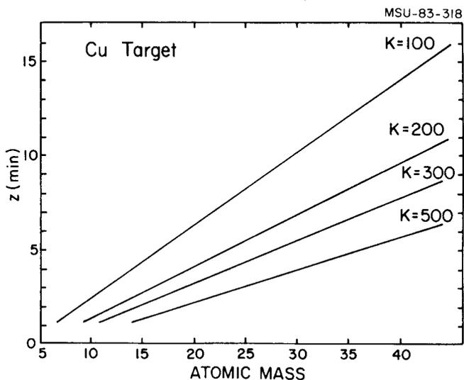
Fig. 2. The minimum charge state (Z), when stripped to (Z+1) that can activate the cyclotron central region, is shown for various cyclotron K factors (MeV) as a function of atomic number with copper used for the Coulomb barrier.
