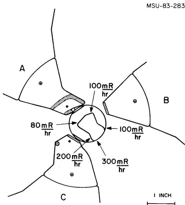
Fig. 1. A median plane cross sectional view of the central region of the K500 superconducting cyclotron is shown. The dees are labeled A, B and C. The ion source is located within the 1-3/8" diameter circle at the center with the source slit opposite of the puller located in dee A. The arrows are indicating measured radiation levels (mrem/hr.) at contact with an ionization chamber after a run with a 30 MeV/u  $^{14}\text{N}^{4+}$  beam.
