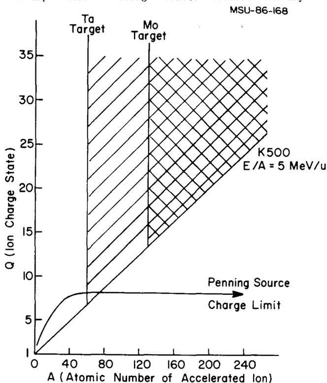
Fig. 3. The accelerated ion charge state versus its atomic number is plotted for the K500 cyclotron. The shaded area is where induced  $\alpha$  activity can occur within the accelerator. The normally obtained Penning ion source charges are below this shaded area.
