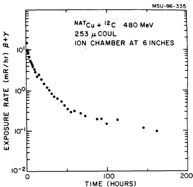
Fig. 4. The decay curve for the irradiation of a copper foil with a 40 MeV/u carbon beam and a total charge collected of 253 microcoulombs.
