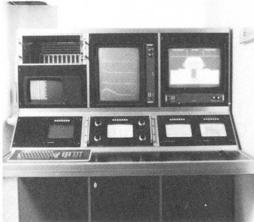
Fig. 2: Control console for the compact cyclotron CP42H -
