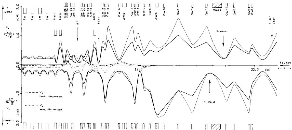
Fig.2: Beam envelopes and dispersion trajectories in TRANSPORT notation for a beam without space charge (thick line) resp. for a beam with 40 mA intensity (thin line).
