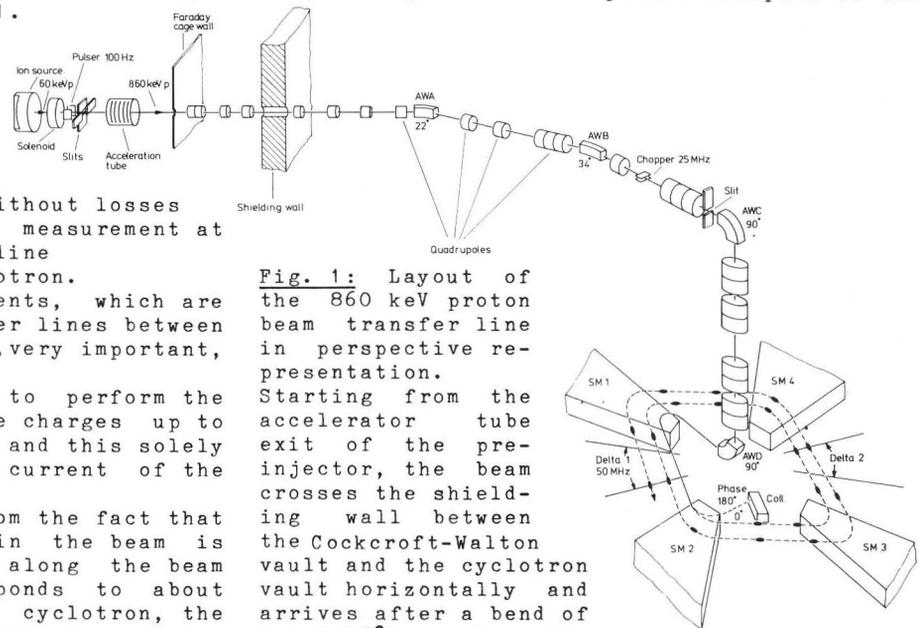
**Fig. 1:** Layout of the 860 keV proton beam transfer line in perspective representation.
