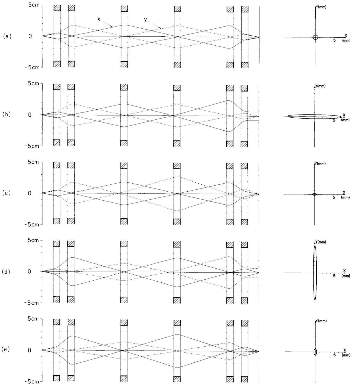
Fig. 3: Beam envelope plots showing an orthogonal quadrupole system with (a) optimum  $x_f$  and  $y_f$ , (b)  $x_f$  increased,  $y_f$  unaltered and (c)  $y_f$  decreased,  $x_f$  unaltered. Reverse quadrupole polarities give (d)  $y_f$  increased  $x_f$  unaltered and (e)  $x_f$  decreased and  $y_f$  unaltered.
