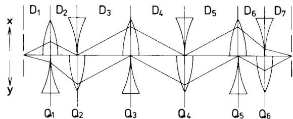
Fig.1: Six quadrupoles (represented as thin lenses) in an orthogonal arrangement.
