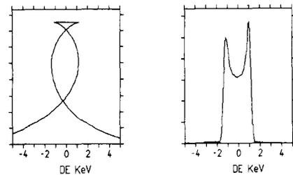
Fig. 9: Top figure shows  $dU/dn$  for same charge density as in fig. 8 but partial compensation with third harmonic  $\epsilon_3 = .113$  and K-value of .06. The lower left figure shows the azimuthal charge density versus energy deviation from central particle. The lower right figure shows the energy spectrum. The energy spread has been reduced to 3.4 keV/turn compared with 20 keV/turn for the uncompensated case.
