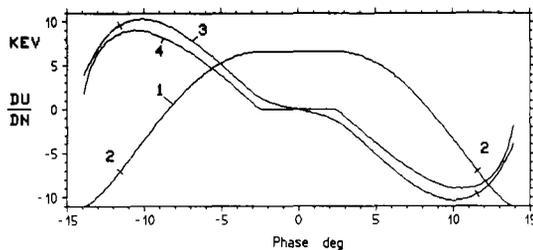
Fig. 8: Voltage gain per turn  $dU/dn$  from longitudinal space charge forces for a 2 mA beam at radius 2300 mm of Injector II at SIN.
