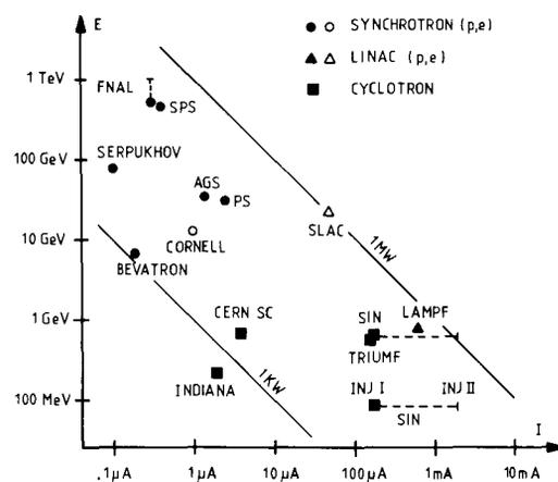
Fig. 1: Energy versus average beam intensity for some medium to high energy accelerators. The two slanted lines indicate points for 1 kW and 1 MW beam power respectively.
