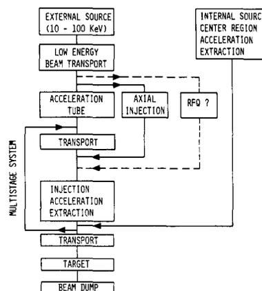
Fig. 2: Structure diagram for cyclotron facilities with internal and external ion sources. RF-quadrupoles (RFQ) are possible future candidates as low energy injectors.
