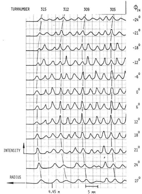
Fig. 5: Demonstration of large phase acceptance of flattop system. Shown are the last 11 out of 315 turns in the SIN ring cyclotron for different injection phases  $\phi_{in}$ . The phase range for single turn extraction is more than  $40^\circ$ . The clear distinction of separate turns for the extreme phases proves the excellent phase stability.
