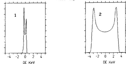
Fig. 10: Charge density and voltage gain  $dU/dn$  for an optimistic case (curves 1) and for a pessimistic case (curves 2) both with a 2 mA beam in the injector II (as in fig. 8). Lower figures show the energy spectra for the two cases with energy spreads of 1 keV/turn and 7 keV/turn respectively. The big influence of the charge distribution in the tails is clearly evident.
