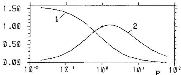
Fig. 4: Geometrical form factors  $g_1(p)$  for curve 1 and  $g_2(p)$  for curve 2 are used to calculate the electric field at the edge of rotationally symmetric ellipsoids. p is the ratio of the longitudinal to transversal diameter. For  $p > 1$  the ellipsoid has a cigar shape.
