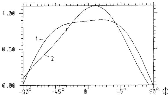
Fig. 7: Accelerating voltage with third harmonic component  $\epsilon_3$ :  $V(\phi) = \cos \phi - \epsilon_3 \cos(3\phi - \phi_3)$ . The parameters are chosen such that at  $\phi_0$  marked by a vertical tick,  $V''(\phi_0) = 0$ .  $K = v(\phi_0) \cdot v'(\phi_0)$  is a current dependent parameter describing the compensation of longitudinal space charge forces.
