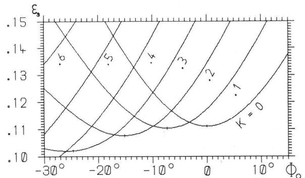
Fig. 6: Compensation of the linear part of the longitudinal space charge forces with a third harmonic RF-component  $\epsilon_3$  and a shift in the central beam phase  $\phi_0$  with respect to the fundamental RF.  $K$  is a dimensionless parameter proportional to the slope of the accelerating voltage at  $\phi_0$ . The optimum  $K$  depends on the detailed shape of the azimuthal charge density and increases proportional to the beam current.
