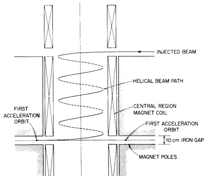
Fig. 1. Elevation view of the injected beam as it enters the central region of the cyclotron. The incoming beam is in a plane parallel to, and 1 m from, the median plane. It is deflected into a helical path, transported to the median plane, and inflected into the first acceleration orbit. The elements that direct the beam into and out of the helical path are not shown.
