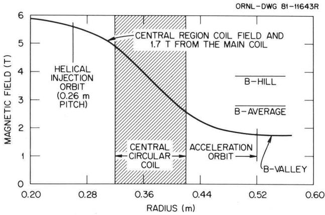
Fig. 2. A central region coil located between the injection orbit and the acceleration orbit provides a field twice that at the acceleration orbit.
