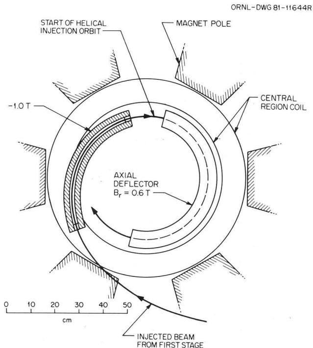
Fig. 3. Plan view of the injection system where the beam enters 1 m from the median plane.
