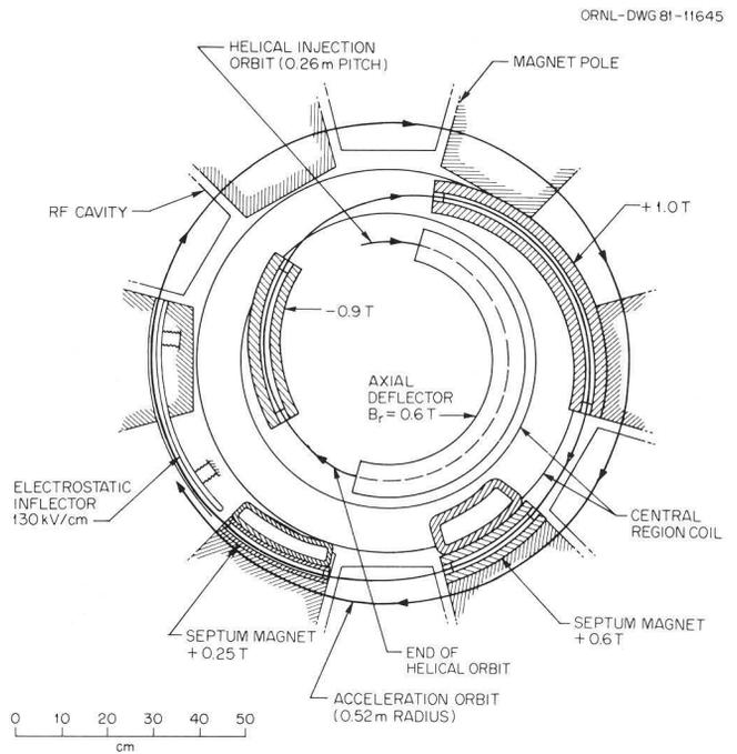
Fig. 4. View at the median plane of the system for deflecting the beam from a helical orbit and inflecting it onto an acceleration orbit.
