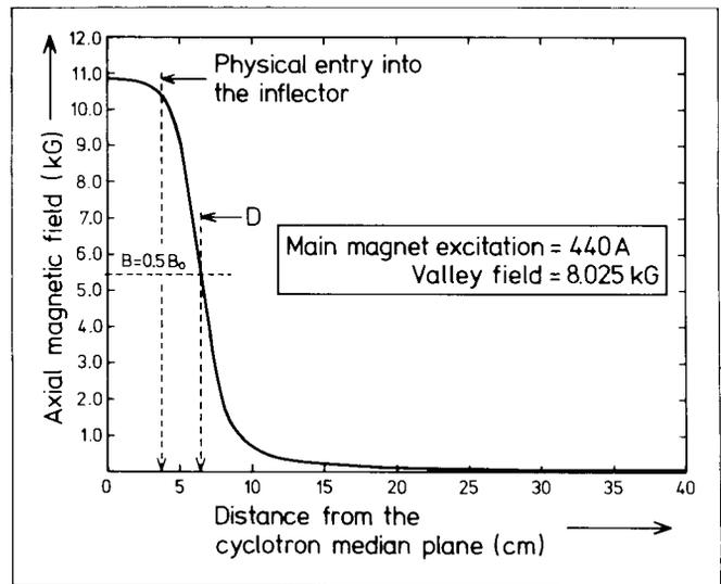
Fig. 3: Magnetic field measured in the axial hole through the cyclotron magnet yoke. Measurements carried out along the axis of the present ion source tube.
