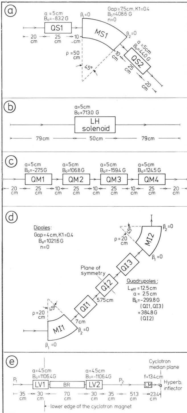
Fig. 2: Configuration and design parameters of a) a unit cell of the 180° bending + charge state analysis system b) a unit cell of the beam transport system of solenoids c) the phase space matching system d) the doubly achromatic 90° bending system and e) the axial injection system. Magnetic field values shown are for a beam of 20.432 kG-cm rigidity (i.e. 5 keV/nucleon and Q/A=1/2).
