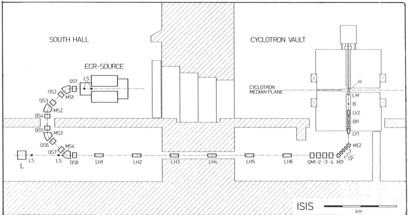
Fig. 1: Layout of the external injection system at JULIC: L-source for light ions upto Helium; LS-spherical lenses; QS, QM, QI-quadrupole magnets; MS, MI-dipole magnets; LH, LV-solenoid lenses, LM-magnetic lens, B-buncher and H-hyperboloid inflector.
