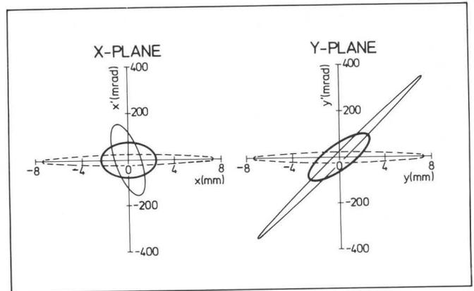
Fig. 6: Phase space ellipses. Dotted lines: at the beginning of the system; thick lines: at the end of the system for zero beam current as well as for the system optimized for  $100 \mu\text{A}$ ; thin lines: at the end of the non-optimized system for  $100 \mu\text{A}$  beam current.
