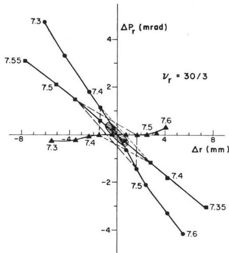
Fig. 2 : The position of the unstable fixed points in the vicinity of the  $\nu_r = 30/3$  resonance which occurs near 7.45 GeV. The dashed triangles connect the 7.42 and 7.48 GeV fixed points, about 2.3 turns on either side of the resonance. Also shown is the anticipated size of the beam ellipse; some particles will experience non-linear or unstable motion for 5 turns.
