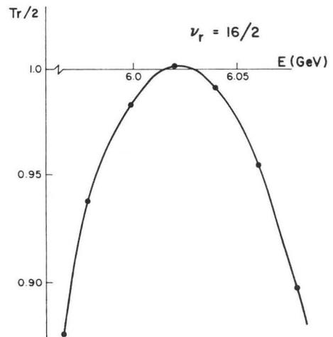
Fig. 4 : The half-trace of the horizontal transfer matrix in the vicinity of the  $\nu_r = 16/2$  resonance when a 16<sup>th</sup> harmonic field gradient  $d(\Delta B_{16}/B)/dR$  of  $3 \times 10^{-5}/\text{cm}$  is superimposed. The motion is unstable for 1 turn.
