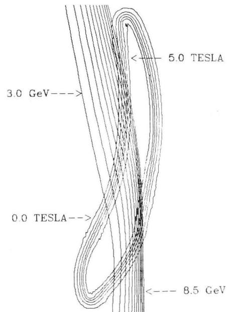
**Fig. 1** : Magnetic field contours and proton orbits computed for the second stage ring cyclotron. The field contours are plotted at 1 T intervals from 0 to 5 T and the orbits at 0.5 GeV intervals from 3 to 8.5 GeV.
