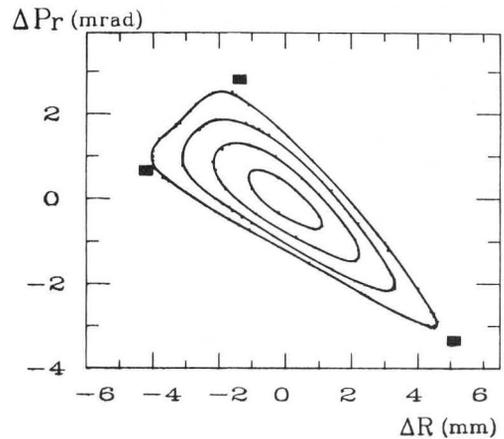
Fig. 3 : Static phase space ( $x, p_x$ ) figure at 7.40 GeV in the vicinity of the  $\nu_r = 30/3$  resonance. Not all turns are shown. ■ = fixed point.
