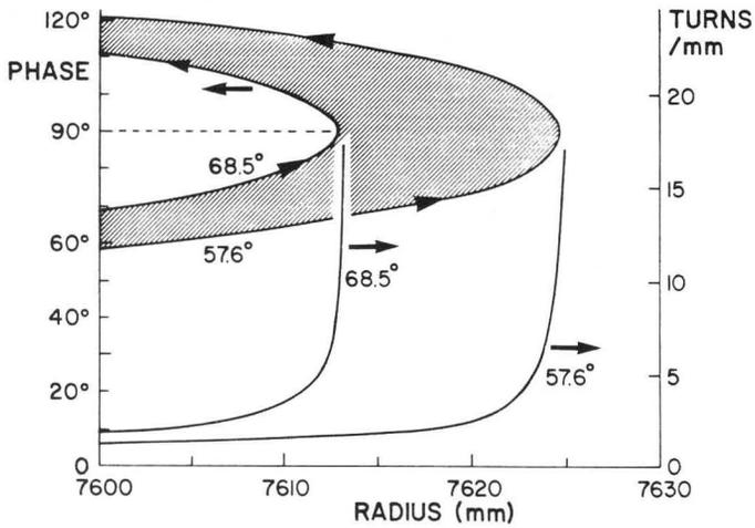
Fig. 5 : The phase history of the ions starting at 57.6° and 68.5° for beam stacking between 7600 mm and 7625 mm radius. All the ions in the cross-hatched area are collected in one packet. The lower curves give the turn density for the two extreme values of the phase.
