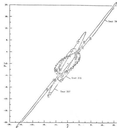
Fig.5: Effects of coupling resonance in the pre-extraction region on vertical beam ellipse.
