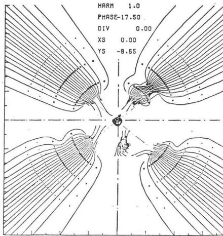
Fig.1: Central region's equipotentials distribution and central trajectory for the fundamental mode.
