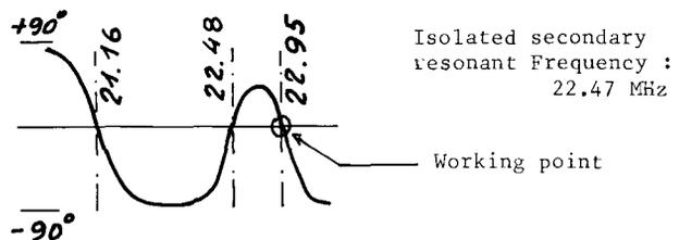
Of course we work near the lower peak with an impedance of about 2000 ohm, which can be easily adjusted when
