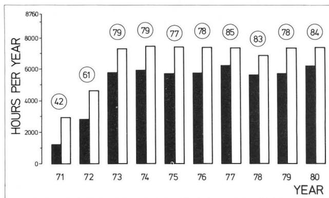
Fig. 3: Operating record of JULIC in the past decade. ■ cyclotron being operational □ scheduled operating time (84) portion of cyclotron being operational with respect to the scheduled operating time in %.
