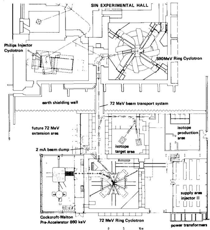
**Fig. 1:** Plan view of the accelerators at SIN. The existing accelerators, a 590 MeV-ring and an injector cyclotron, are shown in the upper half of the drawing. The new injector under construction is a combination of a 860 keV pre-accelerator and a 72 MeV ring cyclotron. The isotope production facility is in the planning stage. A separate building was erected for the new installations.
