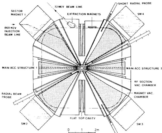
Fig. 4: Plan view showing the main components of the 72 MeV ring cyclotron.
