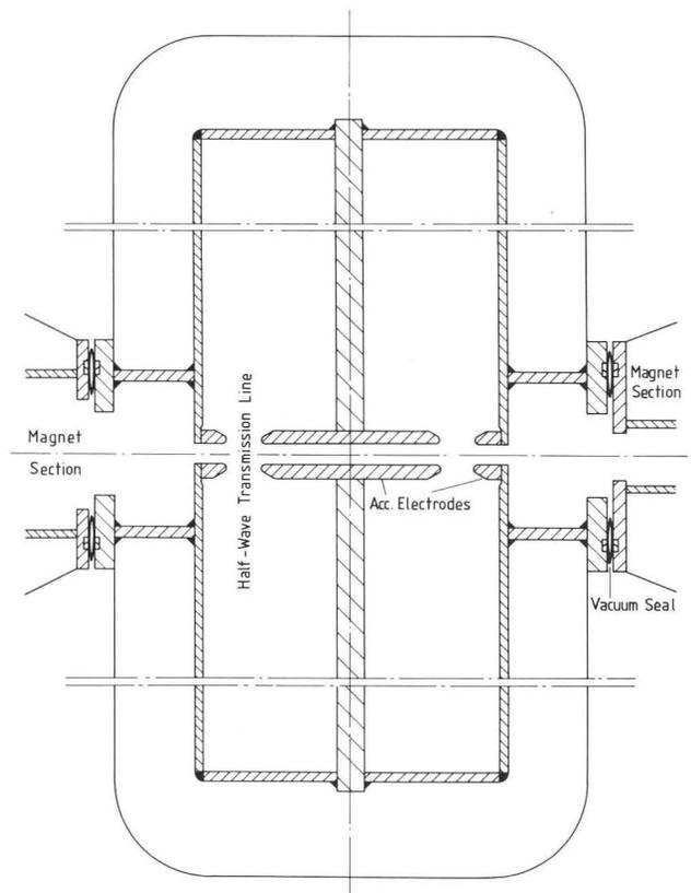
Fig. 12: Cut through a 50 MHz resonator, the main accelerating structure of the 72 MeV ring cyclotron. The accelerating electrodes are located in the voltage maximum of a half wave transmission line. The resonance frequency is adjusted by varying two capacitors between the accelerating electrodes and the chamber wall. The beam aperture is 4 cm.
