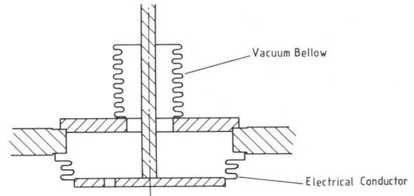
Fig. 15: Sketch of a tuning piston for the 152 MHz flattop cavities. It will penetrate the cavity wall in a location where maximum magnetic RF-field occurs. With a stroke of 1 cm a tuning range of 300 kHz is achieved.
