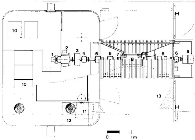
Fig. 3: Dome layout showing the location of the ion source, the 60 keV beam line, the accelerating tube and the auxiliary equipment. 1. Ion source, 2. 2000 l/s turbo pump, 3. Solenoid, 4. Pulser, 5. Iris-diaphragm, 6. Diagnostic elements, 7. Collimator, 8. SF<sub>6</sub> insulated accelerating tube, 9. Quadrupoles, 10. Power supplies, control and auxiliary equipment, 11. Laser data link, 12. Cooling system.
