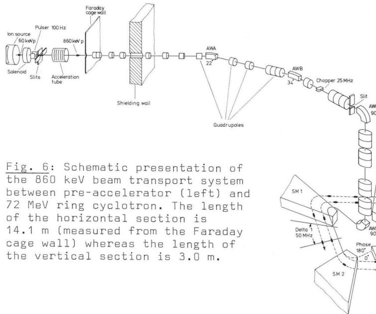
Fig. 6: Schematic presentation of the 860 keV beam transport system between pre-accelerator (left) and 72 MeV ring cyclotron. The length of the horizontal section is 14.1 m (measured from the Faraday cage wall) whereas the length of the vertical section is 3.0 m.
