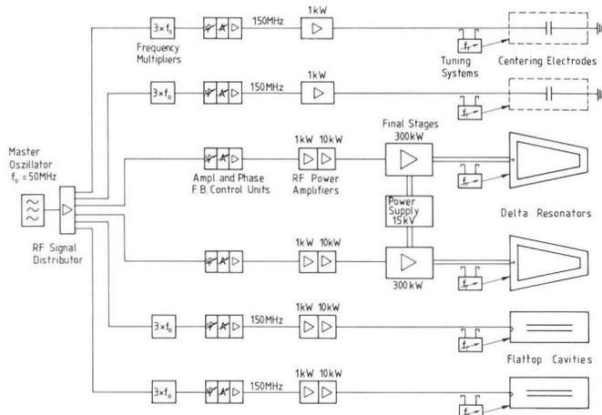
Fig. 11: Block diagram showing the 3 different resonators with its associated amplifier chains. They all have their own amplitude and phase regulation loops (not shown).
