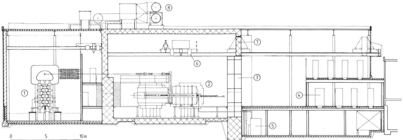
Fig. 16: Longitudinal section through the injector building. 1. Cockcroft-Walton pre-accelerator, 2. 72 MeV ring cyclotron, 3. Shielding wall erected from movable blocks, 4. Power supplies, 5. 50 MHz power amplifier with 50  $\Omega$  coaxial line, 6. Crane 32/3,2 t, 7. Mobile shielding port, 8. Ventilation systems.
