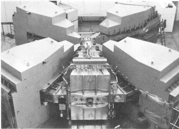
Fig. 7: The 72 MeV ring cyclotron under construction in May 1981. The prototype of the 50 MHz-resonators is installed between two sector magnets. A new Type of inflatable vacuum seals was developed to be used as joints between neighbouring vacuum sections. Vacuum tests which involved the resonator and two magnets demonstrated the excellent performance of the new seals.
