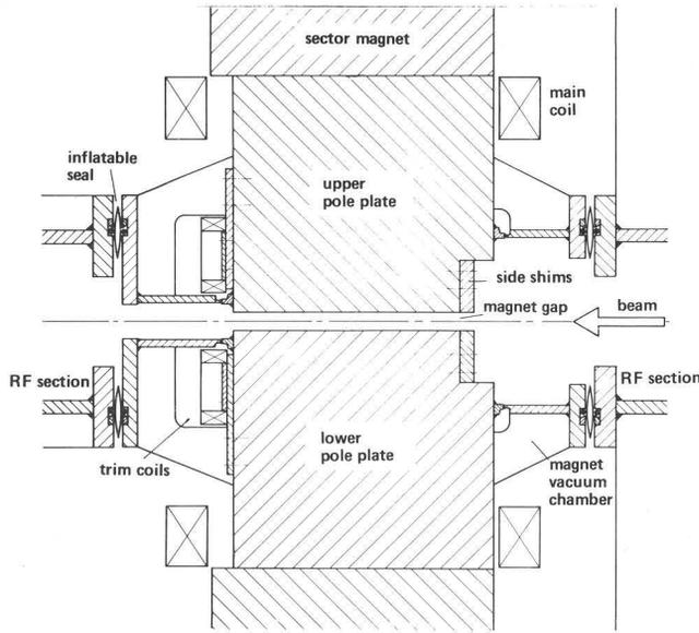
Fig. 8: Cut through a sector magnet showing schematically the pole plates with the main coils, the trim coils and the vacuum chamber. Poleplates, gap spacers and vacuum chamber are connected by welding, thus forming a rigid pole package.
