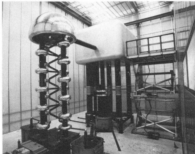
Fig. 2: View showing the main components of the 860 keV pre-accelerator: The Cockcroft - Walton generator designed for 900 kV (left) and the high voltage dome (right) which will house the ion source and the 60 keV beam line. The accelerating tube is not yet installed. A scissors-type lifting platform will provide access to the dome.
