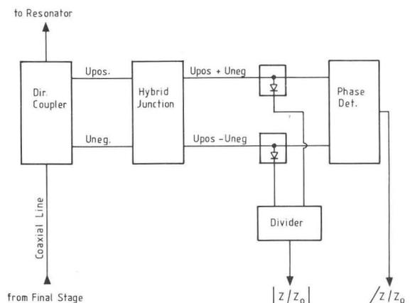
Fig. 14: Block diagram showing the circuit which measures the input impedance of the capacitive coupling system. From phase angle and absolute value feedback signals are derived for the frequency tuning system and for the coupling capacitor. It has to be noted that the beam load exerted on the resonator will have a strong influence on the coupling impedance.
