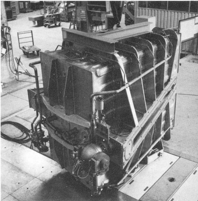
Fig. 13: View showing the first 50 MHz delta resonator. It is made from aluminium. The Q-value is 14'000. The inner conductor and the outside walls will be cooled with demineralized water. The mechanical structure itself is not rigid enough but it needs the additional support provided by the neighbouring magnets when the resonator is under vacuum. Clamps will transmit the tensile forces between the flanges of the resonator tank and the magnet vacuum chamber.
