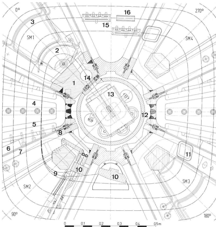
Fig. 5: Center region of the 72 MeV ring cyclotron
