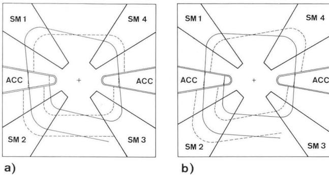
Fig. 10: Orbit deformation in a four sector cyclotron. When the radial gain per turn is large and the 4 sectors are identical, the orbits will deform to a diamond shape as seen in sketch a). The dotted lines represent the equilibrium orbits. (Discontinuities occur in the accelerating gaps as a result of the energy increase). Making sector magnets 2 and 4 wider and magnets 1 and 3 narrower the beam orbits become more regular and the equilibrium orbits will change to a diamond shape.
