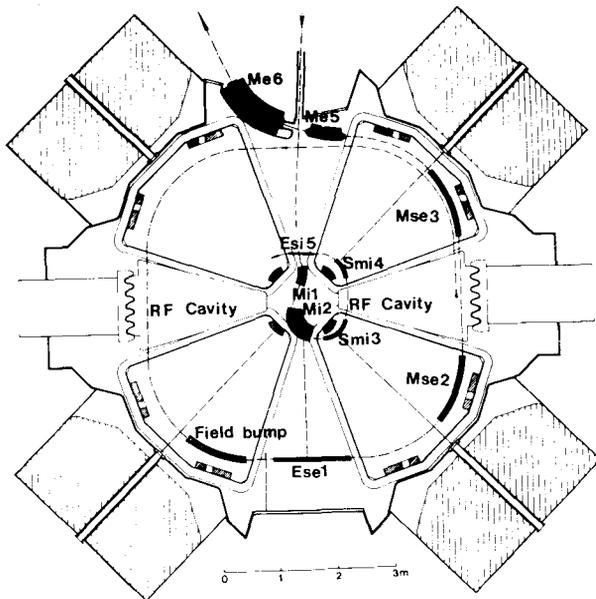
Fig. 9 : Injection and ejection (in SSC1 SMi4, Field Bump are not to be installed.)
