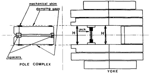
Fig. 5 : Magnet mechanical adjustment.
