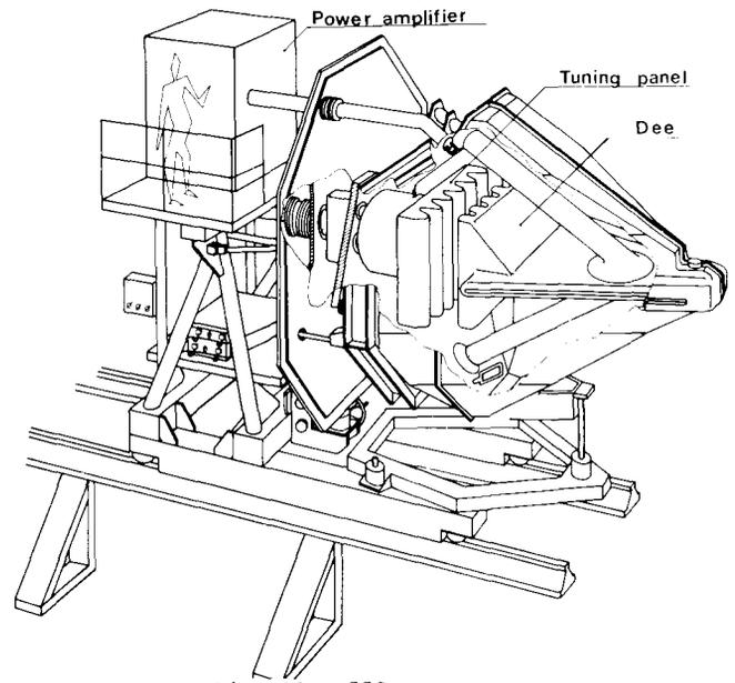
Fig. 10 : SSC resonator.
