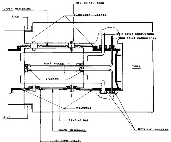
Fig. 8 : Vacuum tightness of the chamber.
