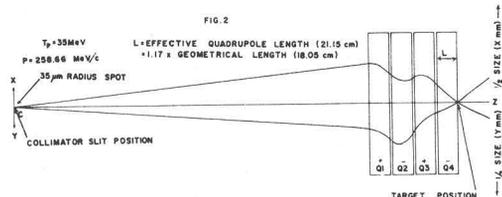
marked. Target scanning can be achieved with the aid of a stepping motor for coarse target displacement (> beam diameter) while a fine scanning of the beam across small portions (≈ beam diameter) of the target can be achieved by a system of electrostatic deflection plates placed inside the fourth quadrupole. Beam parameters at important stages of propagation are tabulated in Table 3. These, together with the data
