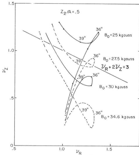
Fig. 8. Operating ( $\nu_R, \nu_Z$ ) plot for an ion with  $Z_2/A = .5$  at different center field levels.
