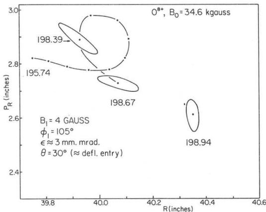
Fig. 16. Turn to turn separation at deflector entrance via excitation of  $\nu_R=1$  resonance.
