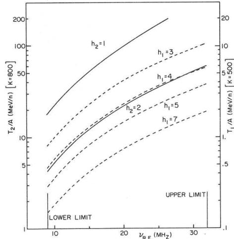
Fig. 9. Energy in MeV/n for both cyclotrons as a function of R.F. frequency for different harmonic modes.
