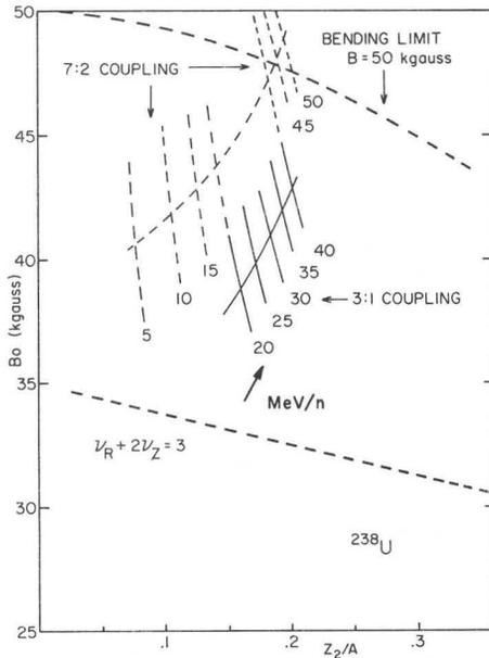
Fig. 11. Operating  $(B_o, Z_2/A)$  plot for uranium. For every HCR the center line refers to the peak charge state, and crosses constant  $T/A$  lines.
