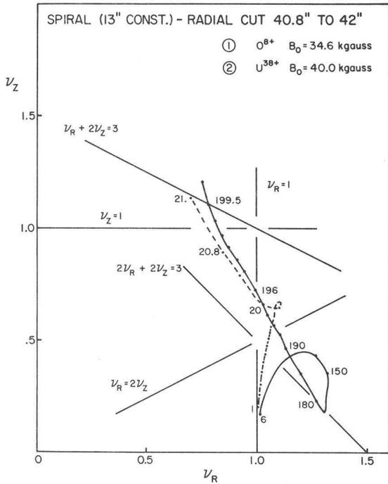
Fig. 7. Operating ( $\nu_R, \nu_Z$ ) plot with a radial cut in the spiral profile from 40.8" to 42". Same ions and fields as Fig. 4.
