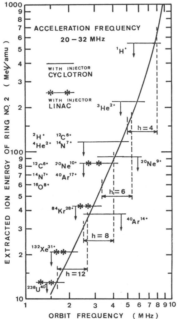
Fig. 7. Acceleration harmonics  $h$  in the two rings for various ions and energies.
