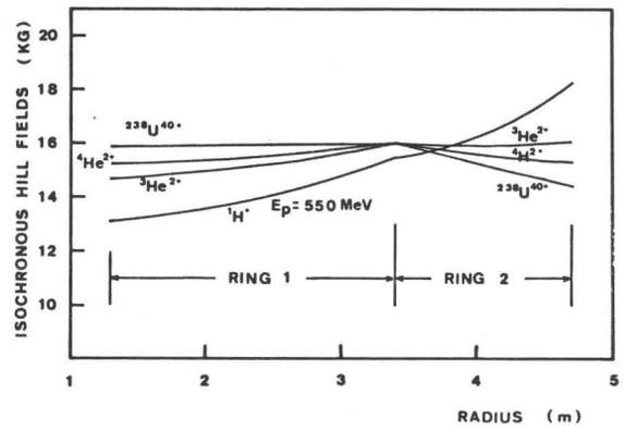
Fig. 6. Isochronous hill field of the ring No. 1 and the ring No. 2 for various ions.
