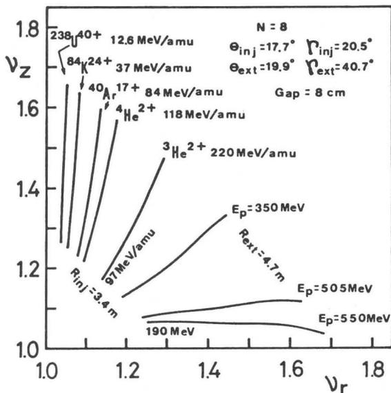
Fig. 5. The radial and axial focusing frequencies for the ring No. 2 calculated with the modified Spy-Ring Code.
