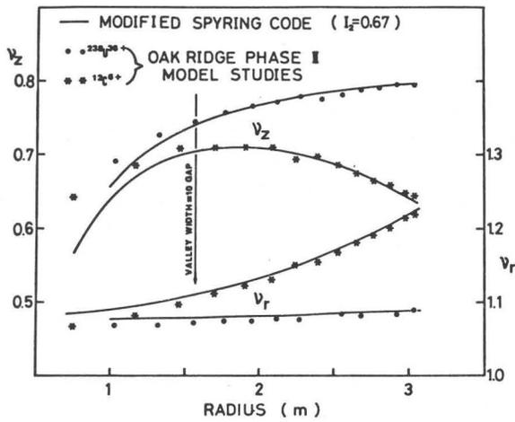
Fig. 3. The radial and axial focusing frequencies calculated with modified Spy-Ring Code and the results of OAK RIDGE PHASE II model magnet study.
