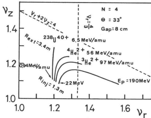
Fig. 4. The radial and axial focusing frequencies for the ring No. 1 calculated with the modified Spy-Ring Code.
