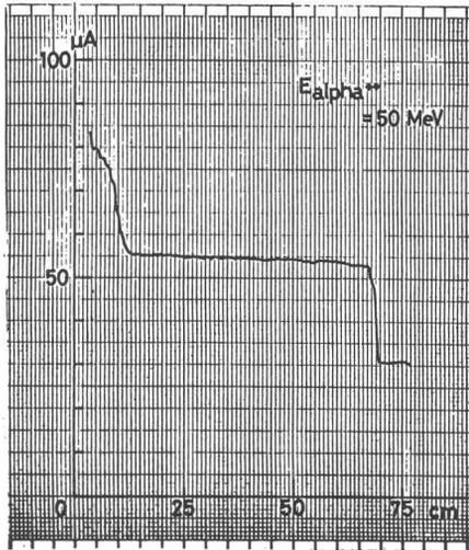
Fig. 5. Radial beam profile of the cyclotron.
