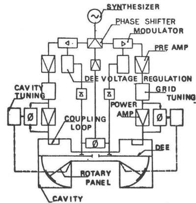
Fig. 3. Radio-frequency circuit diagram.
