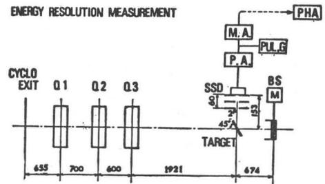
Fig. 8. Method of measuring energy resolution.
