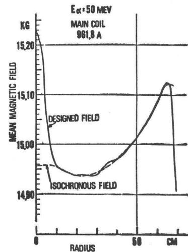
Fig. 4. Magnetic profile of radial direction.
