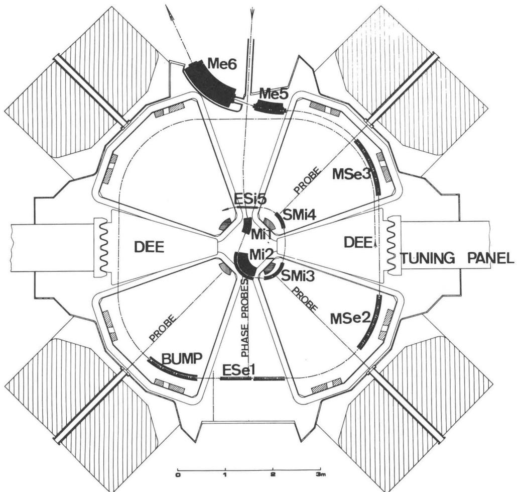
Figure 8. Horizontal cross section of a SSC.
