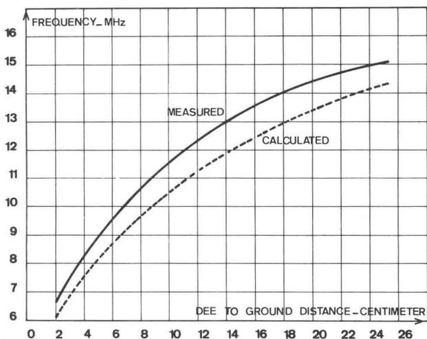
Figure 12. Frequency versus dee to ground distance
