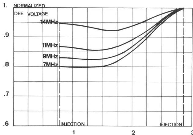
Figure 11. Radial distribution of dee voltage.
