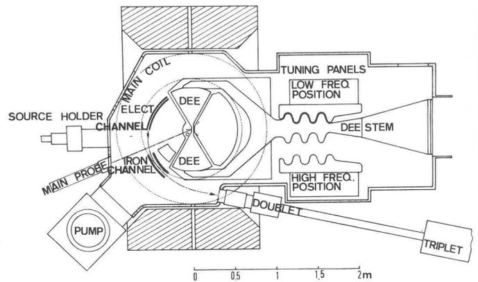
Figure 5. Plan view of the injector cyclotron.
