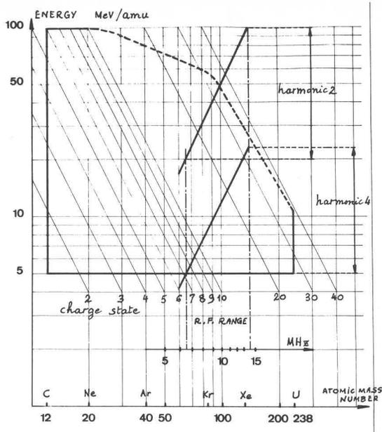
Figure 2. Energy range as a function of atomic mass and charge state.
