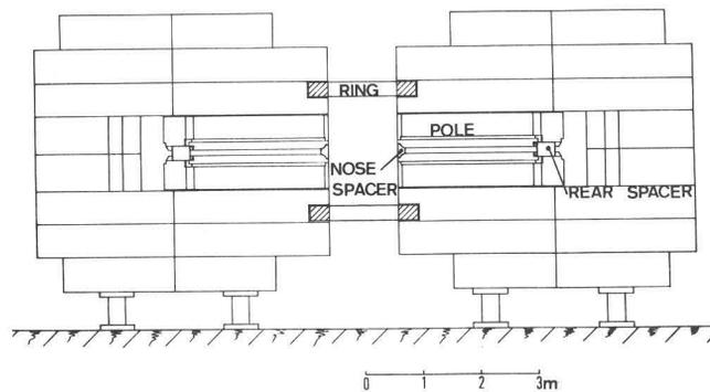
Figure 6. Vertical cross section of two opposite sectors.
