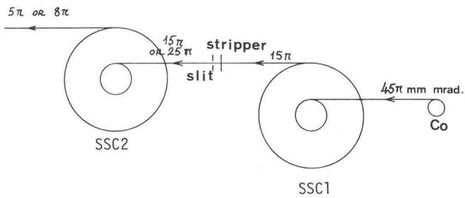
Figure 4. Beam emittances. The emittances are expected to be of the same value in both horizontal and vertical planes.
