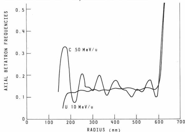
Fig. 4. Axial betatron frequencies for 50 MeV/nucleon carbon and 10 MeV/nucleon uranium. The ripple in the carbon curve is caused by the trim rods. This ripple will be reduced when the azimuthal positioning of the rods is optimized.
