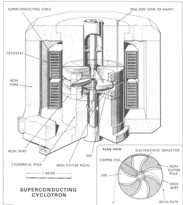
Fig. 2. Current concept of superconducting cyclotron.
