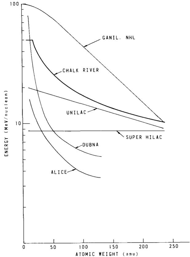
Fig. 1. Comparison of maximum specific energies of some heavy-ion accelerators (existing and proposed).
