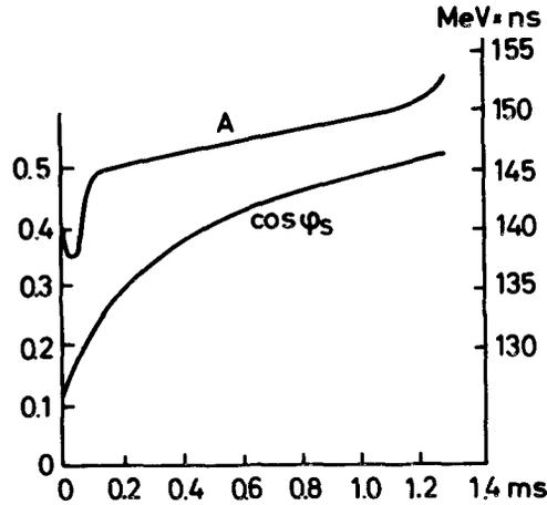
Fig. 4. Bucket parameters for the improved CERN SC. The bucket area  $A$  (right scale) is chosen to increase by 10% over the acceleration period. The resulting  $\cos \phi_s$  (left scale) rises from 0.13 to 0.52. The small minimum in the  $A$  curve stems from the desire to have a smooth  $f(t)$  curve (Fig. 3)
