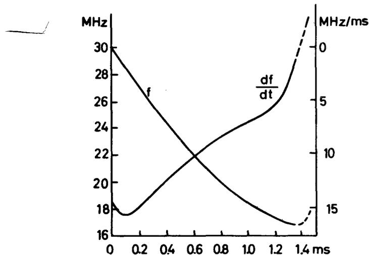
Fig. 3. Frequency vs time function for the improved CERN SC. It is chosen to minimise the acceleration time (1.383 ms)
