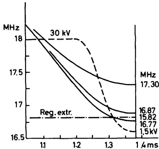
Fig. 5. Details at end of acceleration period showing the nominal rf vs time (lower full curve) as well as frequency (upper full curves) and voltage (dashed curve) functions for adiabatic stacking. The regenerative extraction occurs at 15.82 MHz
