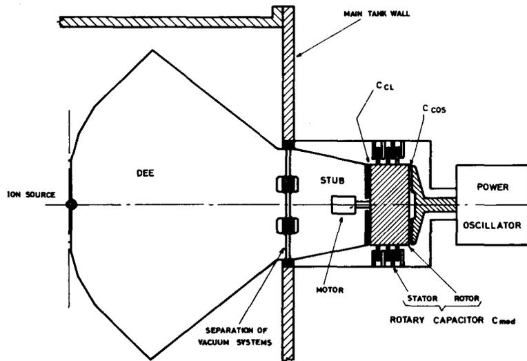
Fig. 2. Principal mechanical arrangement for the new rf system
