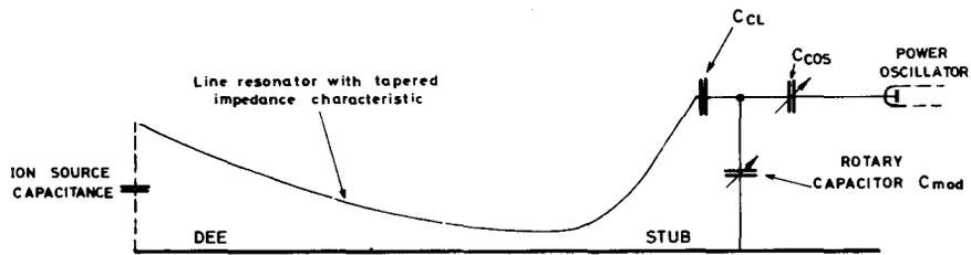
Fig. 1. Principal equivalent circuit for the new rf system
