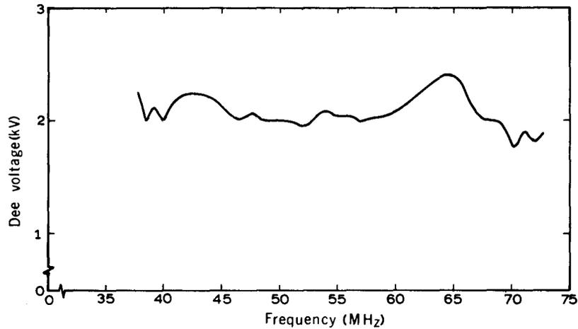
Fig. 5. One-half scale rf model. Measured dee voltage vs frequency
