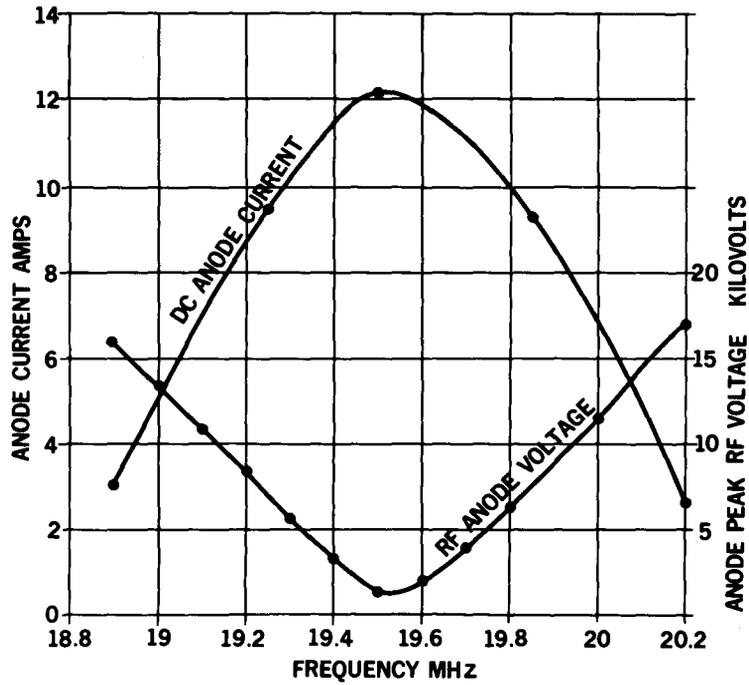
Fig. 7. Broadband cee system. D.C. anode current and rf anode voltage vs frequency. Scaled for 20 kV cee voltage
