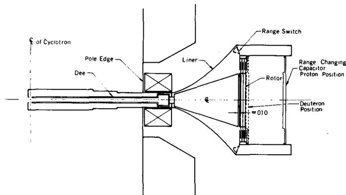
Fig. 2. 184-in synchrocyclotron model rf system. Profile view
