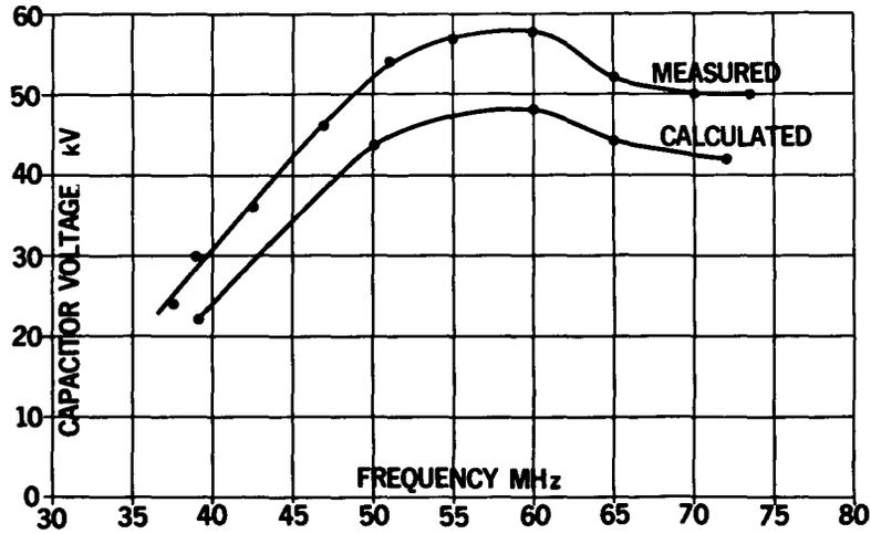
Fig. 3. Computed and measured capacitor voltage vs frequency. Scaled for 40 kV on the dee lip
