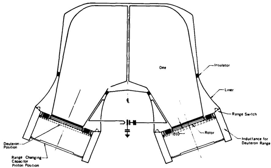
Fig. 1. 184-in synchrocyclotron model rf system. Plan view
