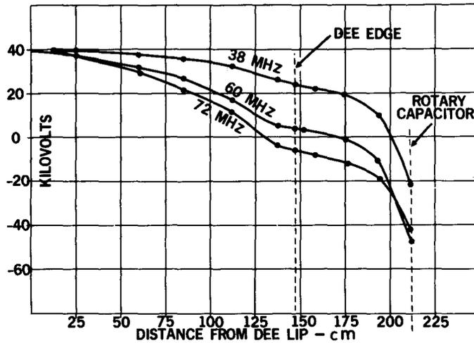
Fig. 4. One-half scale rf model. Voltage vs distance from the dee lip
