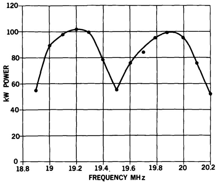
Fig. 8. Broadband cee system. Input power vs frequency. Scaled for 20 kV cee voltage
