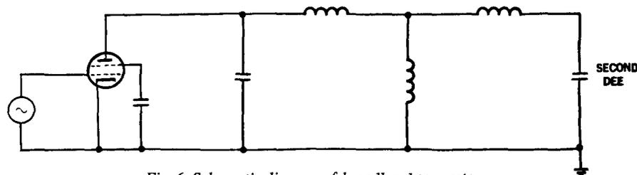
Fig. 6. Schematic diagram of broadband cee system
