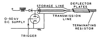
Fig. 11. Time-of-flight beam deflection circuit (schematic)
