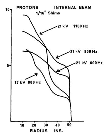
Fig. 5. Variation of internal beam with radius
