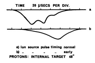
Fig. 9. Variation of time structure with ion-source timing
