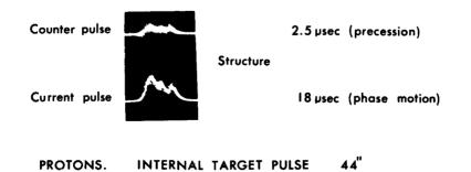
Fig. 7. Time structure of beam striking internal target
