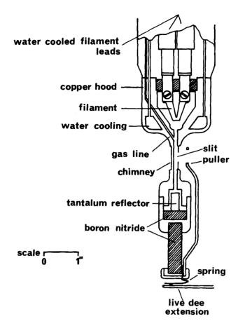
Fig. 3. Hot cathode calutron ion-source
