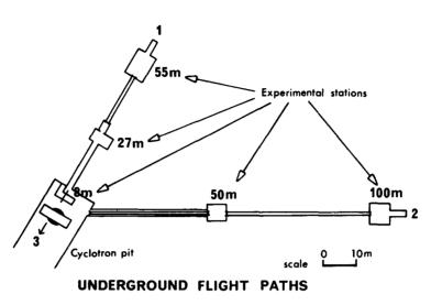
Fig. 12. Layout of neutron flight paths
