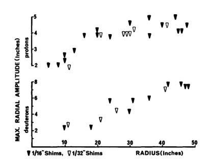
Fig. 8. Estimated maximum radial oscillation amplitude as function of radius
