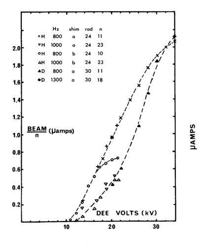
Fig. 6. Variation of internal beam with dee voltage
