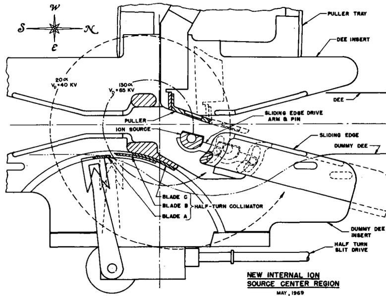
Fig. 7. New internal ion source centre region plan view, showing beam trajectories for lowest and highest energy beams. Note sliding edge on dummy dee insert, moved by pin on anode
