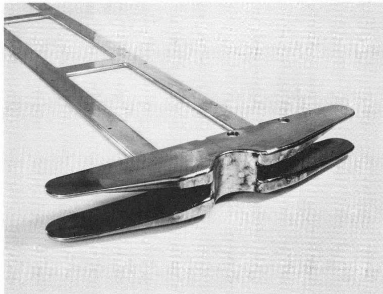
*Fig. 6. Dee insert for axial injection mounted on its tray. Material is inconel*
