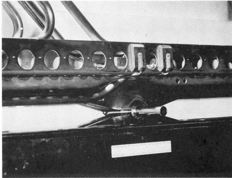
*Fig. 5. Photo of axial injection centre region when set up prior to installation, showing dummy dee with insert, inflector, and dee with insert*
