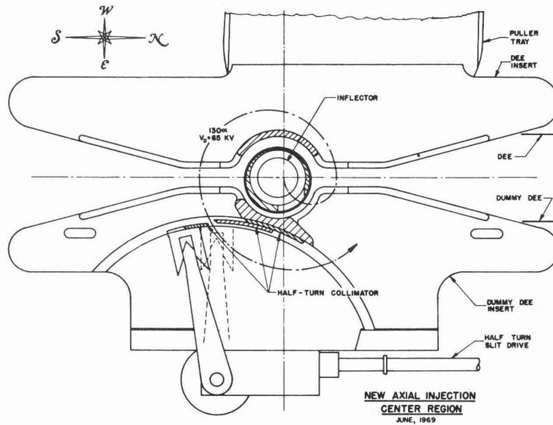
Fig. 4. Axial injection centre region plan view, showing smallest beam trajectory for maximum energy  $\alpha$ -particles. 'Plug-in' dee and dummy dee inserts are shown
