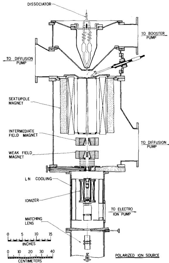
Fig. 1. Polarised-ion source schematic cross-section, showing principal components and vacuum pump ports
