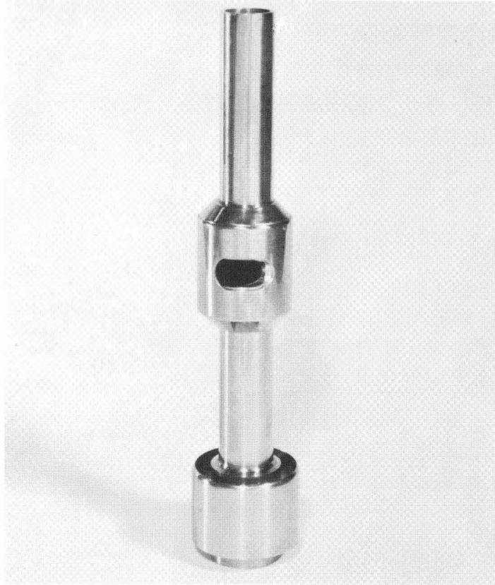
Fig. 3. Inflector housing. Exit slot at centre brings beam into dummy dee. Material is inconel
