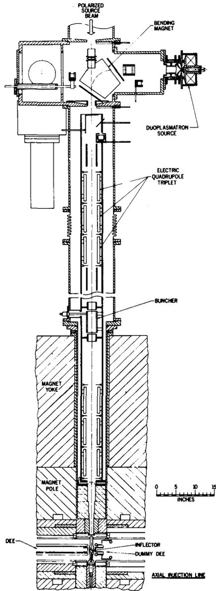
*Fig. 2. Axial injection transport line schematic cross-section, showing components. Note that one quadrupole triplet lens has been omitted*
