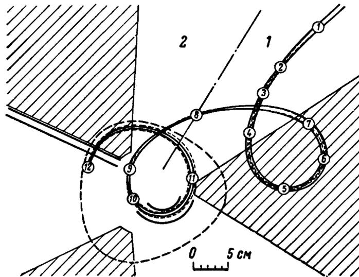
Fig. 13. Lebedev radial injection centre region, showing channel inflector
