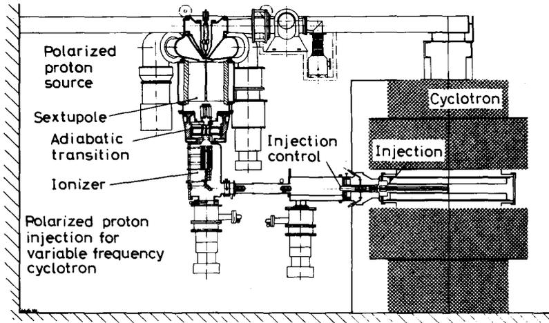
Fig. 15. New Saclay radial system for injecting polarised ions into AVF cyclotron
