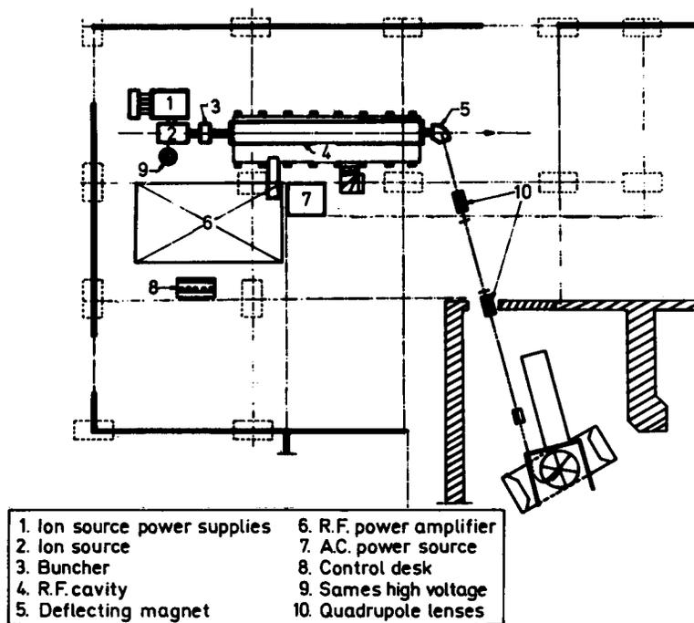
Fig. 19. Orsay heavy-ion radial injection from a linear accelerator
