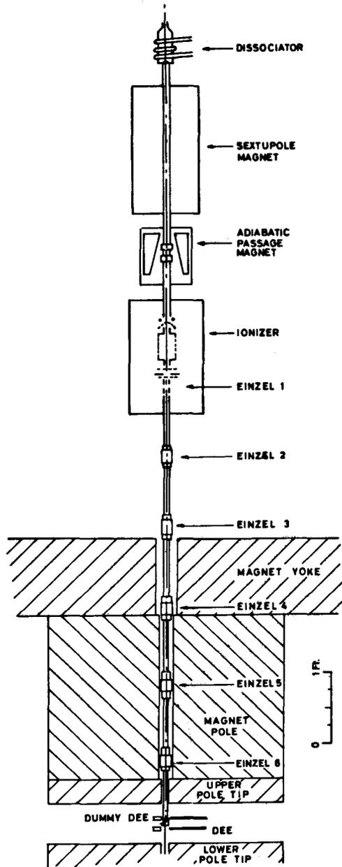
Fig. 4. Birmingham axial injection system for polarised deuterons
