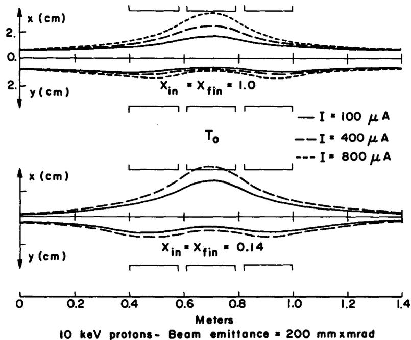
Fig. 11. Beam envelope calculation, including space charge, through Berkeley quadrupole triplet
