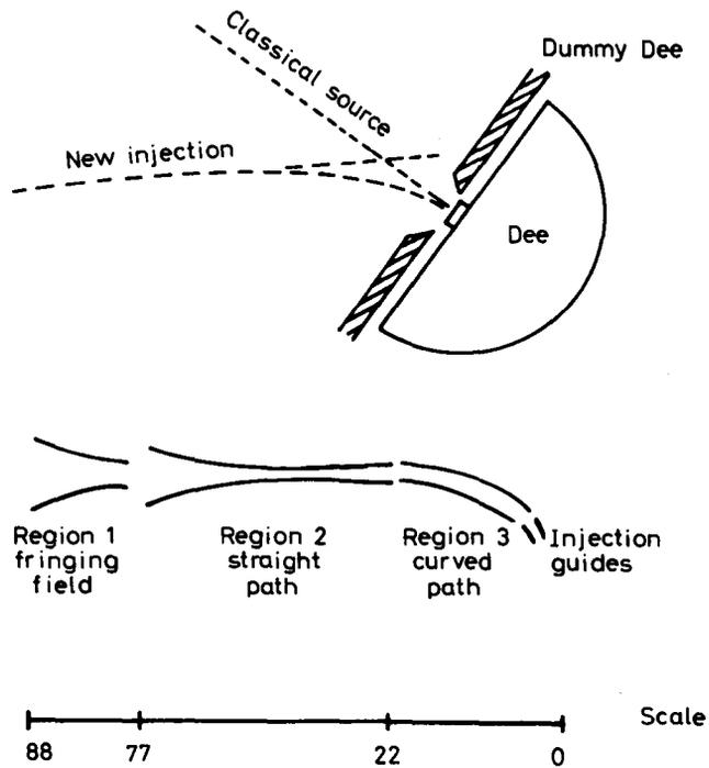
Fig. 16. Schematic layout of new radial ion injection at Saclay
