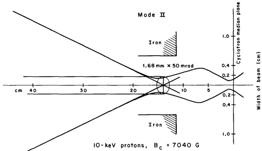
Fig. 9. Beam envelope calculation in ' $\lambda$ -mode' through 'hole-lens' in Berkeley axial injection system
