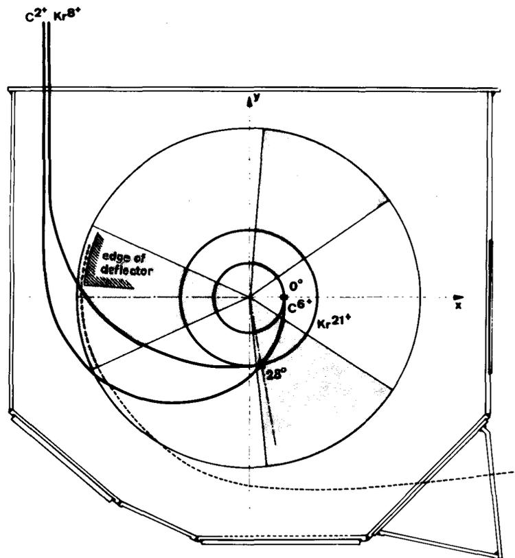
Fig. 20. Orsay centre region, showing heavy ions from linac being stripped, to bring them into a centred orbit
