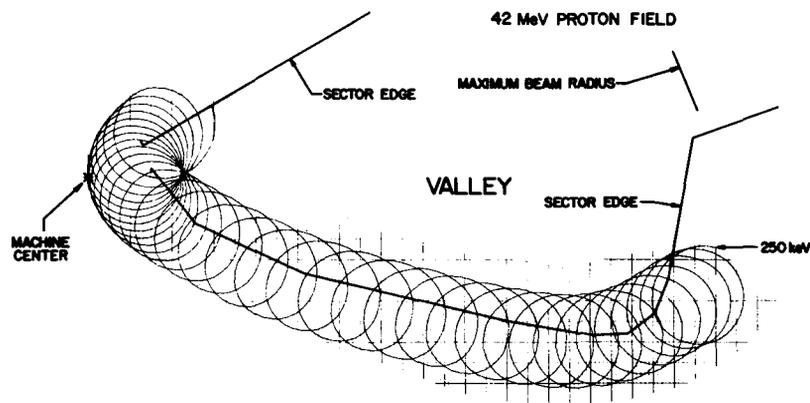
Fig. 14. Michigan State calculated trochoidal injection at 250 keV. Inflector is not designed yet
