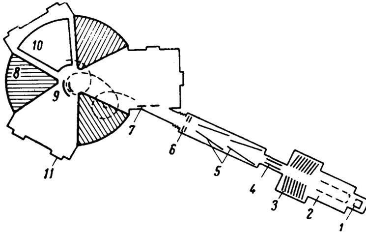
Fig. 12. Radial trochoidal injection in median plane at Lebedev Institute, Moscow
