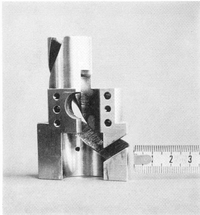
*Fig. 8. Photo of Grenoble channel type electrostatic inflector for axial injection*
