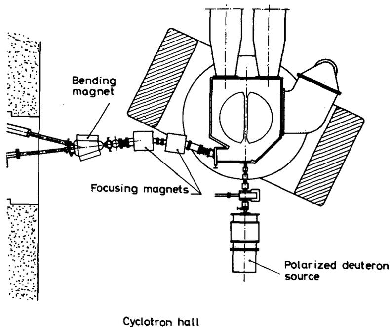
Fig. 2. Plan view of Saclay classical cyclotron showing polarised deuteron source used to inject atomic beam in median plane
