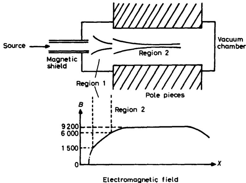
Fig. 17. New Saclay injection system, showing magnetic field behaviour
