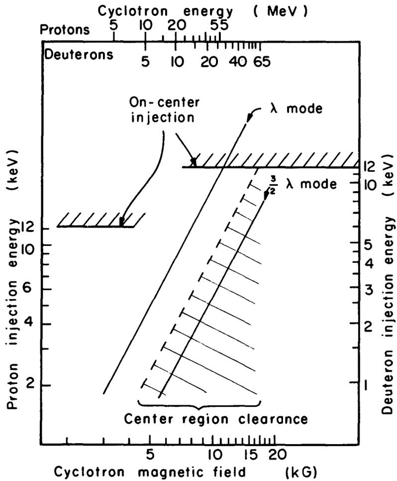
Fig. 10. Regions of allowed (unshaded) operation, and mode lines for Berkeley system
