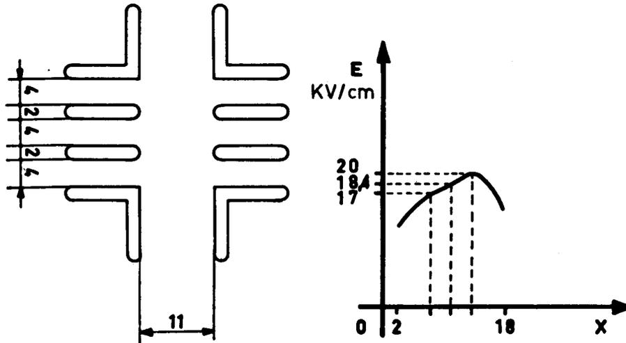
Fig. 18. Electrodes to produce an electric field which cancels magnetic field
