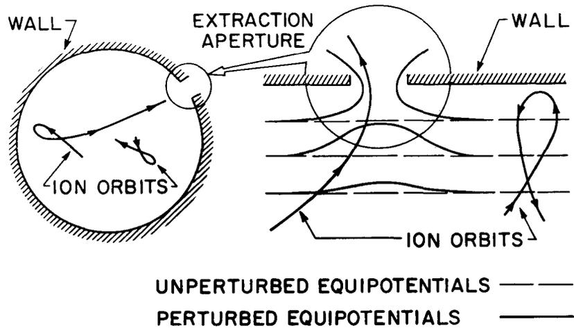
*Fig. 3. Conceptual equipotential configuration and particle trajectories near the extraction aperture of a HIPAC Ion Source. The unperturbed equipotentials arise from the space charge of the electron cloud. The indicated perturbation of these potentials is produced by a suitable arrangement of biased electrodes and/or grids.*
