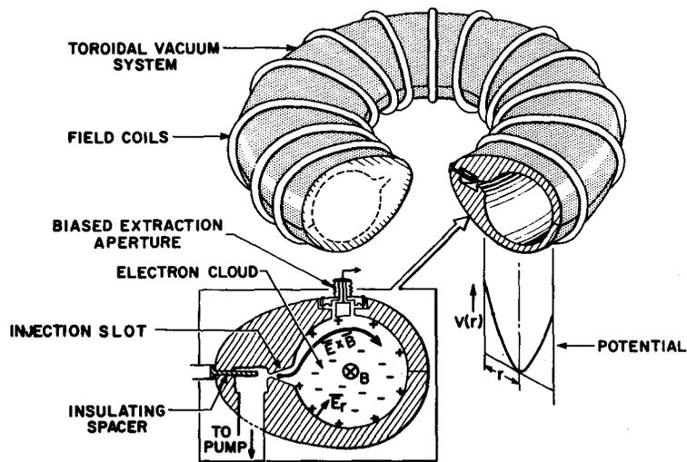
Fig. 1. Conceptual configuration for a HIPAC Source of highly stripped heavy ions
