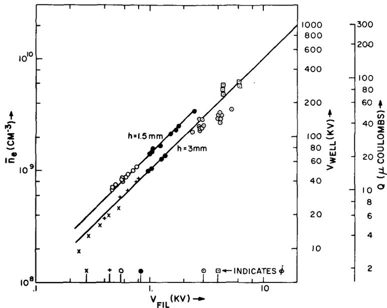
Fig. 8. Experimental results from a torus similar to the one sketched in Fig. 1, having a minor radius of 10 cm. The dependence of  $\bar{n}_e$  on  $V_{fil}$  and  $h^{1/2}$  is apparent.  $\Phi$  is the induced e.m.f.  $\Phi = d/dt (\pi a^2 \bar{B})$ . The directly measured quantity<sup>7</sup> is the total charge  $Q$ ;  $\bar{n}_e$  and  $V_{well}$  are inferred.
