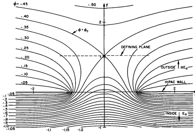
Fig. 5. Two dimensional equipotentials in the vicinity of the extraction aperture. Note the null point in the electric field, caused by the opposition of the HIPAC electric field and the extraction electric field. Ions having energies allowing them to reach equipotentials between the null point and the HIPAC wall can be extracted through the aperture
