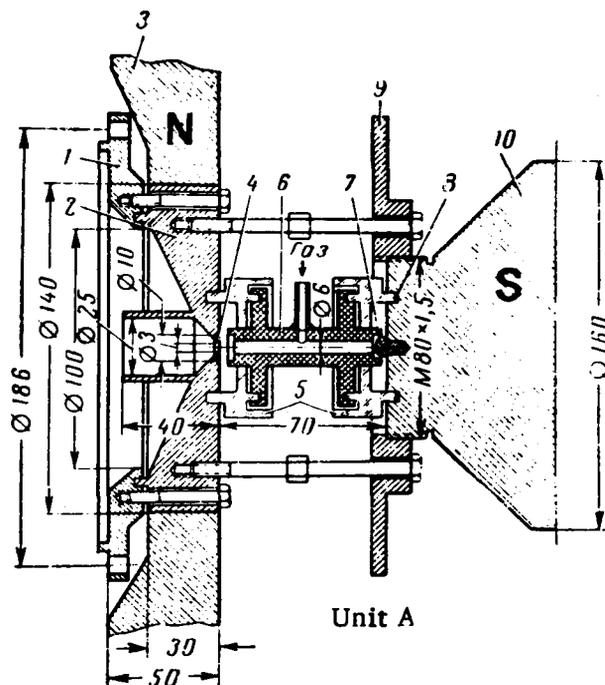
Fig. 4. Cold Cathode P.I.G. Source with End Extraction. The source developed by Mineev and Kovpik<sup>12</sup> used plasma expansion for initial focusing of the ion beam. 3 and 10 – Poles of Electromagnet, 6 – Anode, 5 – Insulator, 7 – Cathode, 4 – Cathode with hole to allow expansion of plasma into the cup
