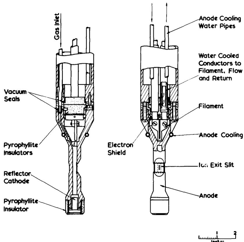
Fig. 1. Floating Cathode P.I.G. Source. This source<sup>3</sup> is a close copy of the Berkeley 88 in cyclotron source developed by Ehlers<sup>4</sup> and used for a short time in the Harwell Variable Energy Cyclotron
