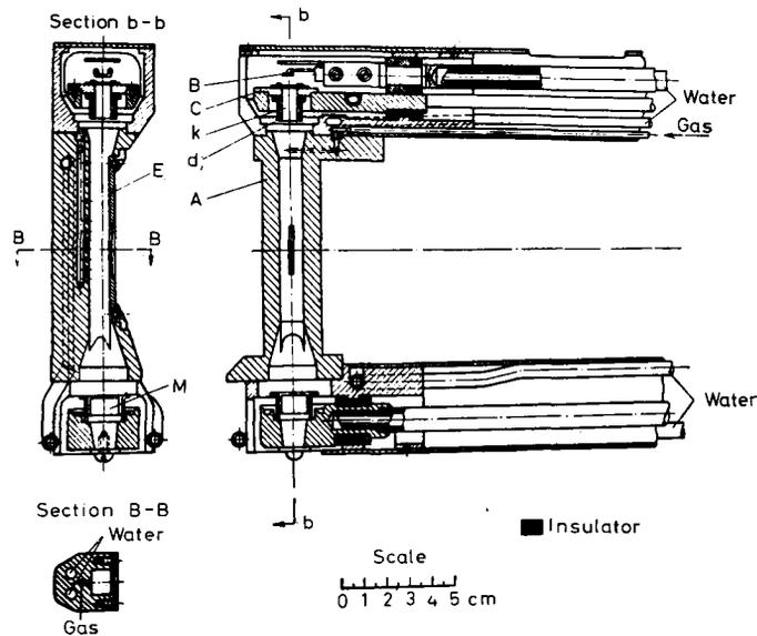
Fig. 2. Indirectly Heated Hot Cathode P.I.G. Source. The figure shows the source originally developed by Morozov, Makov, and Ioffe.<sup>9</sup> A – Anode, k – Cathode, B – Filament for indirect cathode heating
