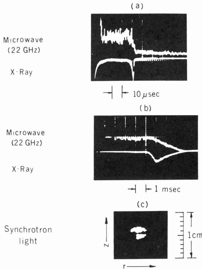
Fig. 16. Diagnostic information on the ERA is obtained. Synchrotron light shows the radii of the ring cross-section to be a few mm. The ring studied here is stable for more than 5 ms
