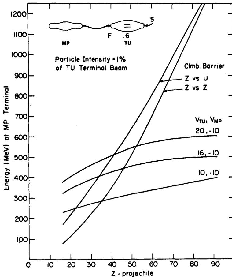
Fig. 13. The energies of heavy ions in the HILAB arrangement are shown for different possible operating potentials. For a 20 MV terminal potential,  $Z = 40$  heavy-ions can penetrate the Coulomb barrier for uranium.
