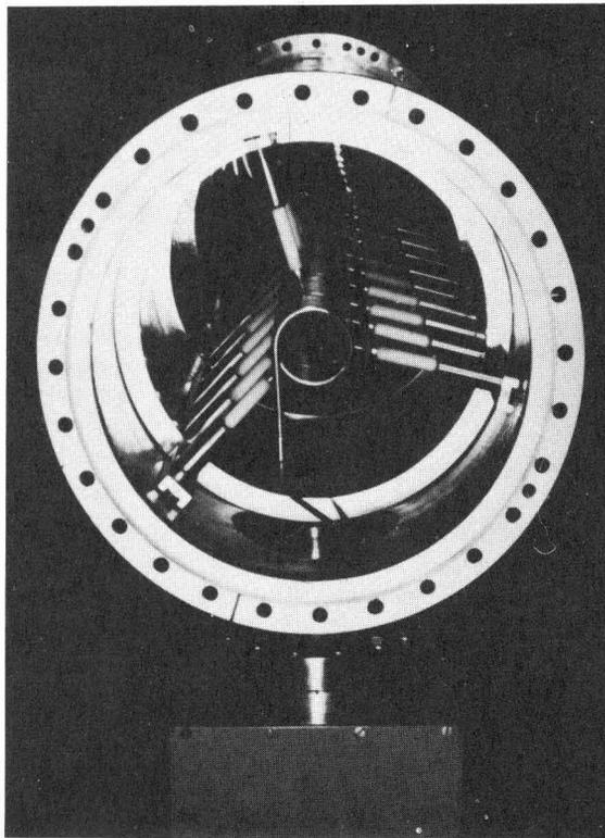
*Fig. 9. A photograph showing the HELAC structure placed in its outer cylindrical casing*
