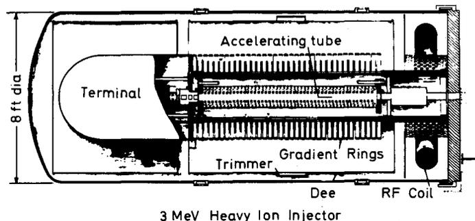
Fig. 6. A section of the d.c. injector for the superHILAC. Not shown in this sketch is a planned 'pressure lock' to enable fast source changes in the terminal without disturbing the pressurised system
