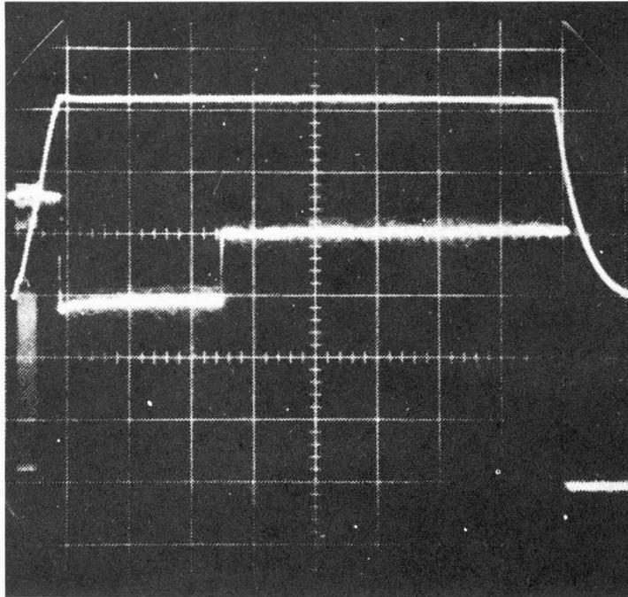
*Fig. 20. Oscilloscope traces showing effect of regulating circuits as a  $50 \mu\text{A}$  beam comes on. The field probe signal trace is at the top, the klystron input power at the bottom*
