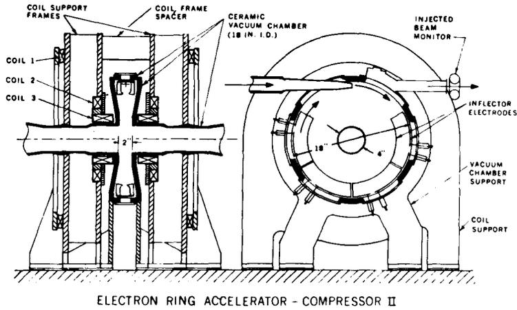
Fig. 14. A sketch of an electron ring apparatus studied at Lawrence Radiation Laboratory. After injection of an intense beam of electrons in a weak magnetic field, additional coils are activated and the energy of the trapped electron ring increases
