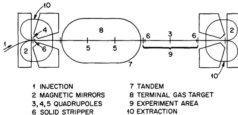
Fig. 17. A sketch of the basic features of the charge-change method of accelerating heavy ions
