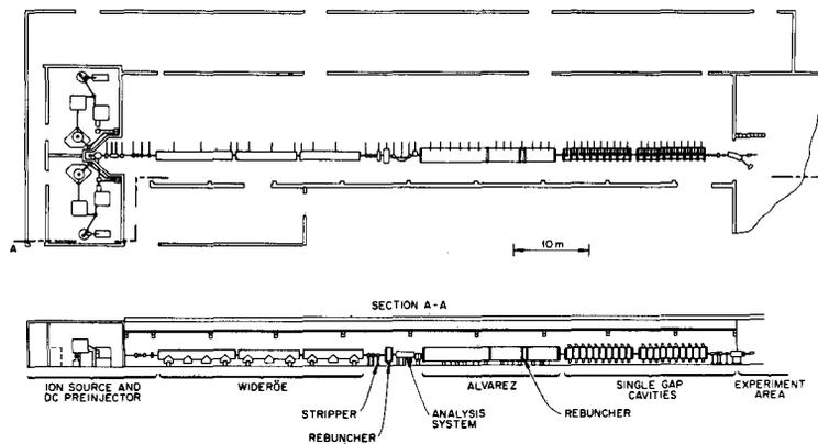
*Fig. 10. A sketch of the system proposed for the UNILAC. It consists of four basic elements: injector, Wideroe linac, Alvarez linac, and a series of single gap separately phased cavities*
