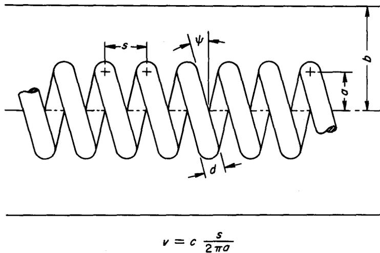
Fig. 7. A sketch of the spiral conductor which is the key to the HELAC concept
