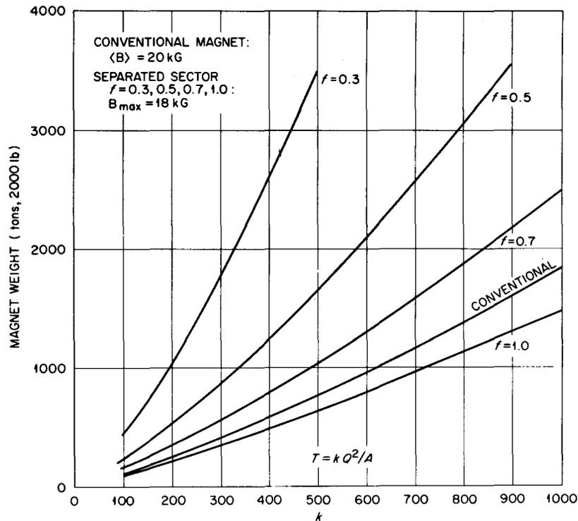
Fig. 4. This is an extension of Fig. 3 in which the lower portions of the scales have been expanded. These magnets would be applicable for cyclotrons using highly stripped ions
