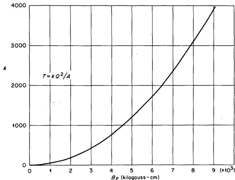
Fig. 1. The size of a cyclotron may be expressed conveniently by a number  $k$  from the formula  $T = kQ^2/A$ , where  $T$  is the kinetic energy of the particle,  $Q$  is the charge state, and  $A$  is the atomic mass number. The relation between this constant,  $k$ , and the magnetic-field-radius product is plotted
