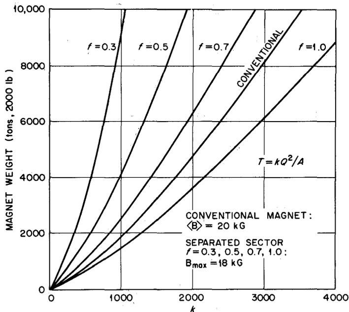
Fig. 3. Magnet weights have been calculated for various size cyclotrons. The f values refer to the fraction of the magnet circumference which is occupied by pole pieces and magnetic field. The lower f values are required to produce necessary focusing for protons and other relativistic particles. The f = 1.0 is for reference only as a lower limit. Lack of access would prevent such a magnet from being practical
