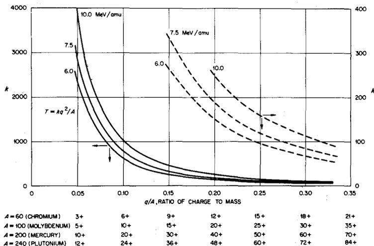
Fig. 2. The size of cyclotron necessary to produce heavy ions of various desired energies. The scale at the bottom gives examples of ions of various masses with different hypothetical charge states to illustrate the different regions of possible design and operation. The dotted lines are for an expanded scale for smaller cyclotrons using very high (Q/A)'s
