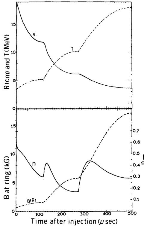
Fig. 15. The sequence of operations in the electron ring accelerator are analysed. Over a 500 μs period, the field is raised to about 17 kG, the radius of the ring decreases to 3.5 cm and the electron kinetic energy increases to 18 MeV
