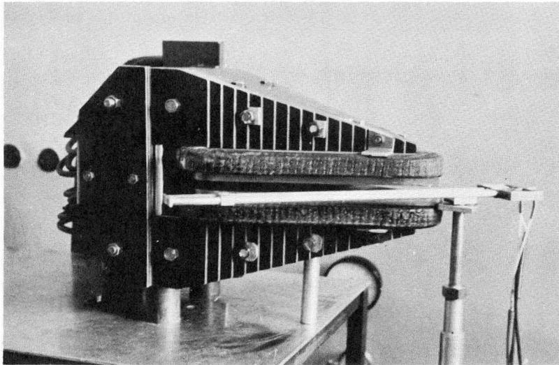
Fig. 1. General view of the sector electromagnet (1: 10 scale) with the Hall detector displacement equipment inside
