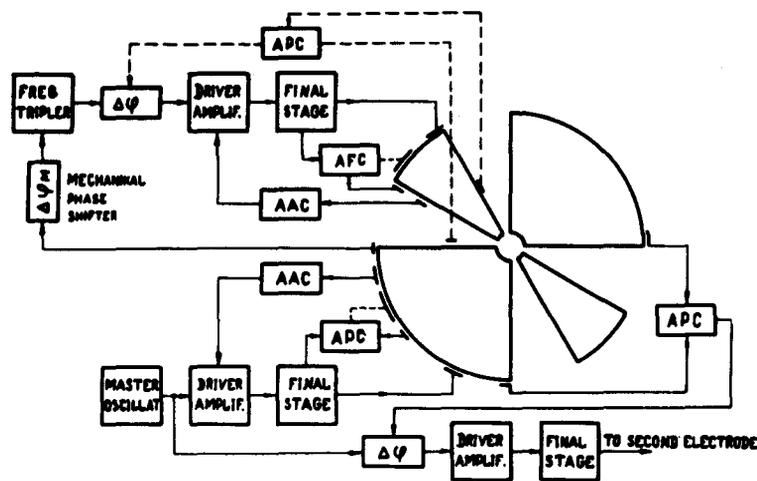
Fig. 3. Block-diagram of the rf supply
