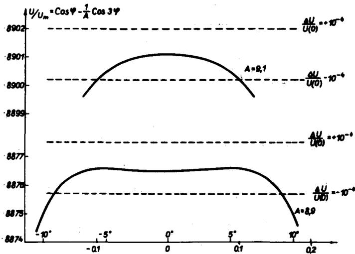
Fig. 2. The values of the equivalent accelerating voltage for various ratios  $U_1/U_3$
