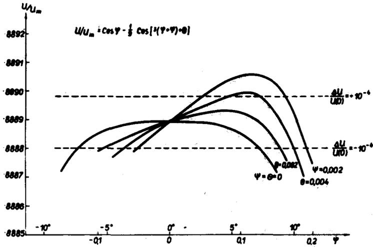
Fig. 1. The values of the equivalent voltage for various phase relations between  $U_1$  and  $U_3$
