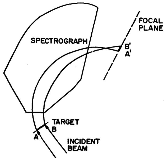
Fig. 5. Dispersion matching. If energy on target increases from B to A image width  $A'B'$  will be reduced
