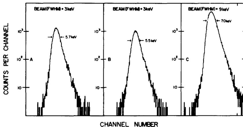
Fig. 6. Spectra are  $^{209}\text{Bi}(p, p)$  with  $E_p = 5.83 \text{ MeV}$  measured at spectrograph focal plane with position sensitive counter. Spectra A and B were taken with 3 keV beam and divergence limits of  $\pm 3 \text{ mr}$  and  $\pm 1 \text{ mr}$  respectively; spectrum C with 9 keV dispersed beam incoherent to 3 keV
