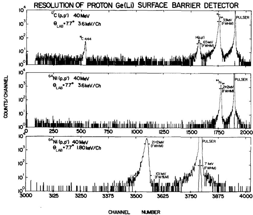
Fig. 4. Spectra of protons inelastically scattered from a  $^{64}\text{Ni}$  target. The incident proton energy is 40 MeV
