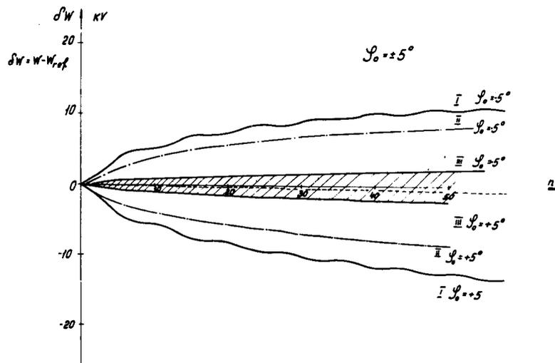
Fig. 2. Energy spread  $\delta W$  (n) for different versions of accelerating systems in ring cyclotrons
