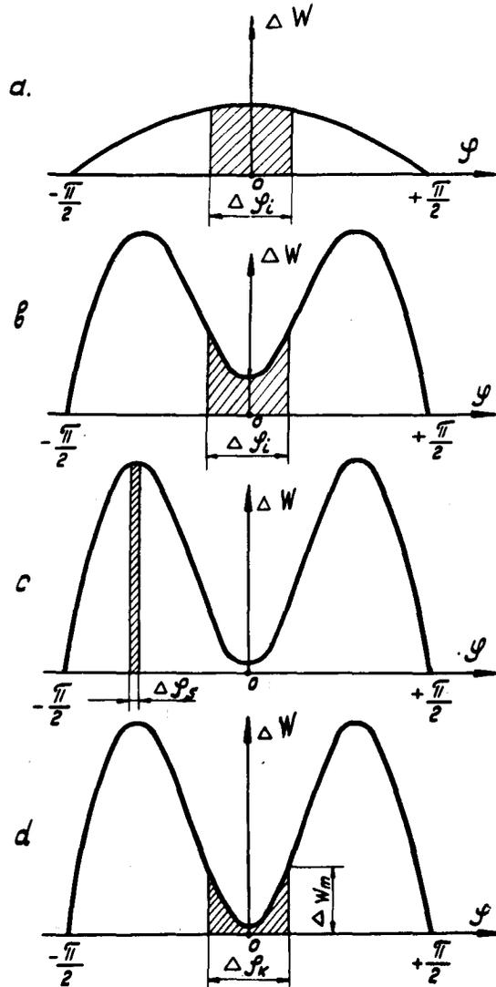
Fig. 4. Scheme of phase motion: (a) First half-revolution; (b) Initial region; (c) Main stage of acceleration; (d) Stage of beam extraction
