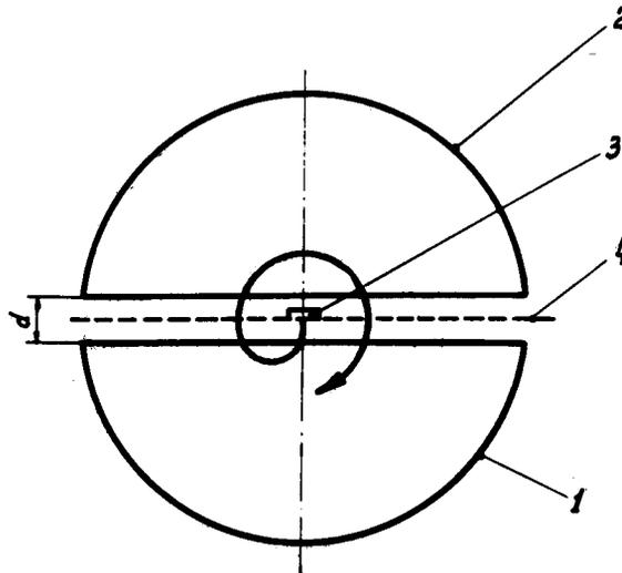
Fig. 3. Simplified scheme for a cyclotron: (1) Main dee; (2) Supplementary dee; (3) Source; (4) Screening frame
