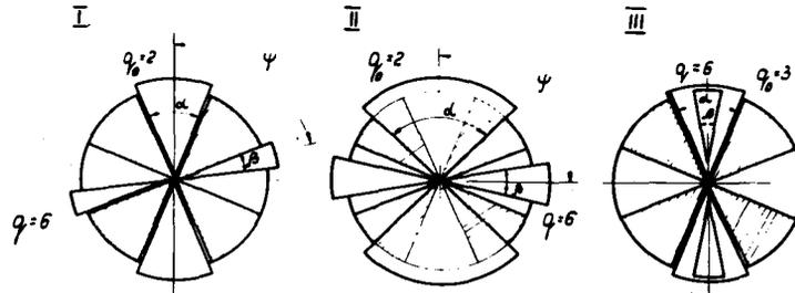
Fig. 1. Schemes for accelerating systems in isochronous cyclotrons, intended to give beams with small energy spread
