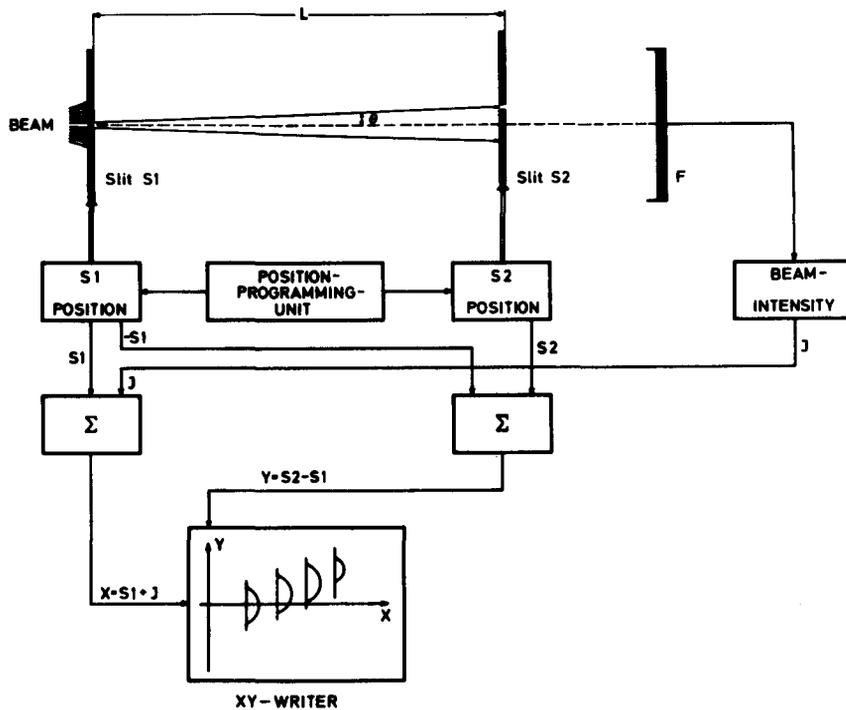
Fig. 1. Principle of the emittance-measuring device (EMA) ( $L$ : drift length;  $F$ : Faraday cup;  $S1, S2$ : position signals of slit  $S1, S2$ ;  $J$ : beam intensity)
