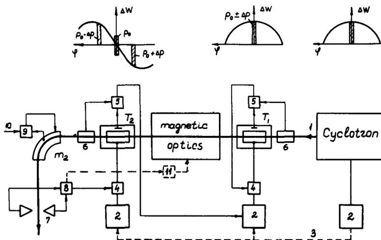
Fig. 4. Block-diagram of the energy variation and stabilisation system.
