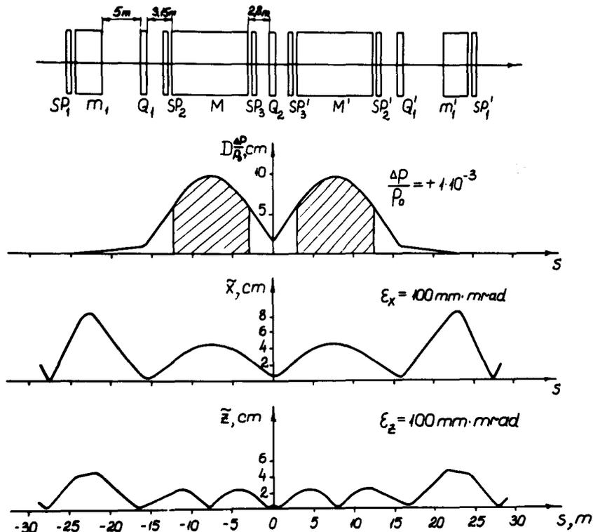
Fig. 3. Dispersive trajectory and beam envelopes
