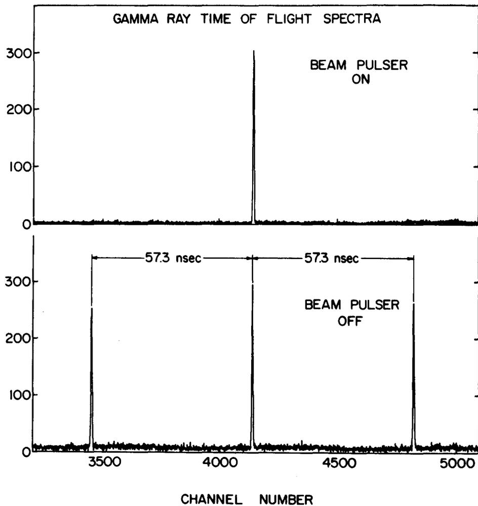
Fig. 6. Time spectrum of gammas produced by protons striking an external target. Upper figure with the pulser on; lower with the pulser off. Pulse shape discrimination was used to eliminate neutron background
