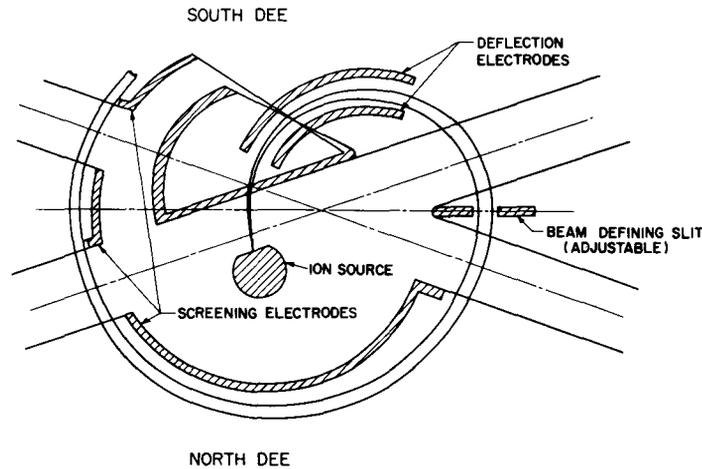
Fig. 1. Plan view of dees, dummy dees, one-half turn beam defining slit, ion source, puller and deflection plates
