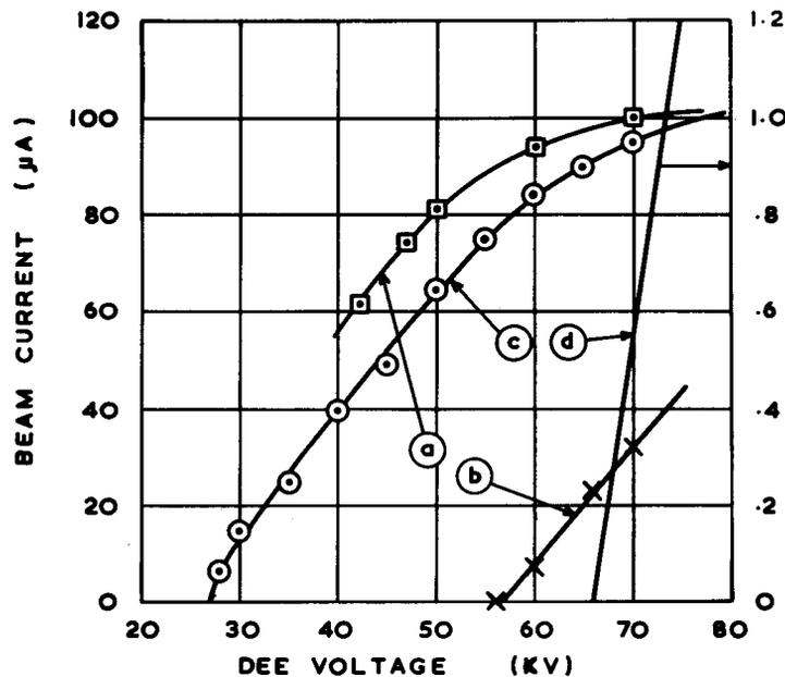
Fig. 3. Beam current vs dee voltage for various harmonic modes
