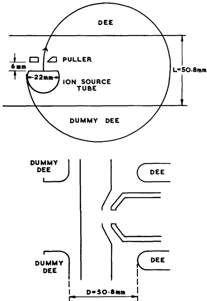
Fig. 2. V.E.C. centre geometry
