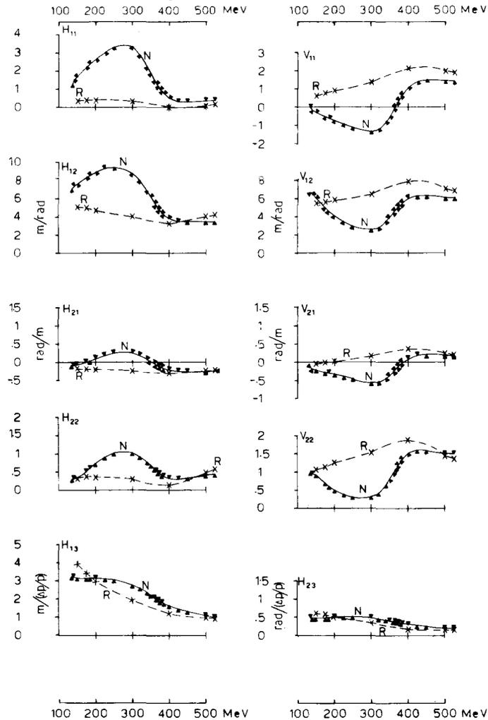
Fig. 2. Transfer matrix elements in the horizontal ( $H_{ij}$ ) and vertical ( $V_{ij}$ ) planes as a function of energy for ions accelerated in the normal direction ( $\Delta$ ) and reverse direction ( $x$ )
