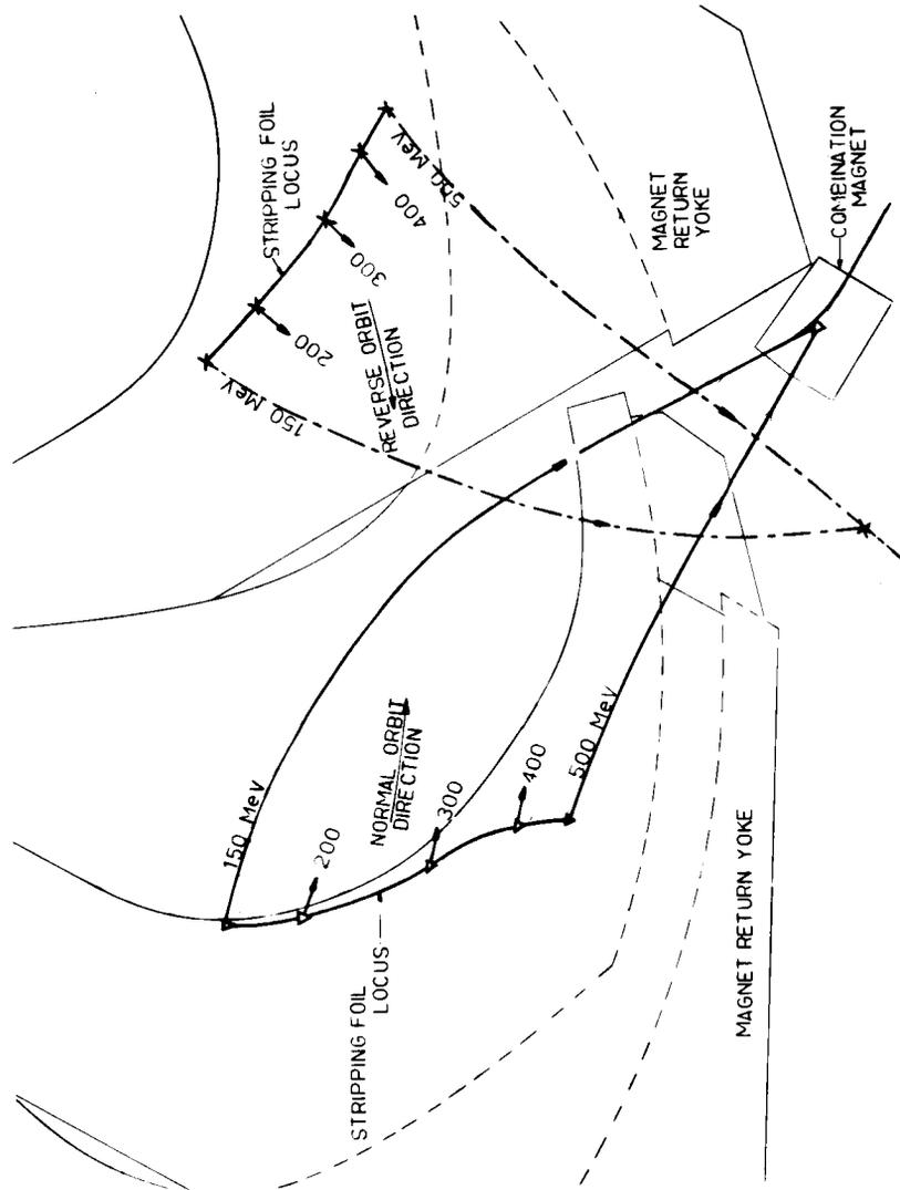
Fig. 1. Stripping foil loci and extraction trajectories for ions accelerated in the normal direction ( $\Delta$ ) and reverse direction ( $x$ )
