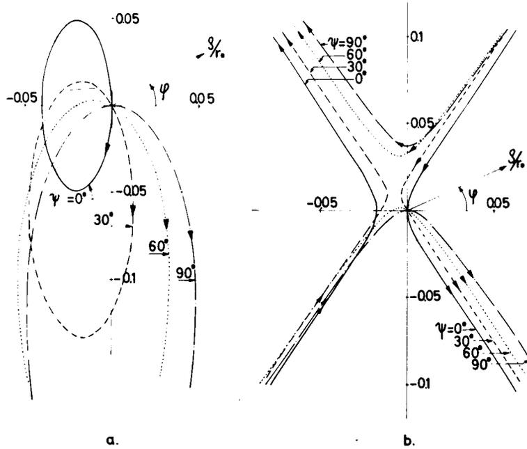
Fig. 1. Orbit centre paths under the influence of first and second harmonic field components.  $\psi$  is the angle of the first harmonic.  $C_0 = 190 \times 10^{-4}$ ,  $C_1 = 13 \times 10^{-4}$ . (a)  $C_2 = 135 \times 10^{-4}$ , (b)  $C_2 = 540 \times 10^{-4}$
