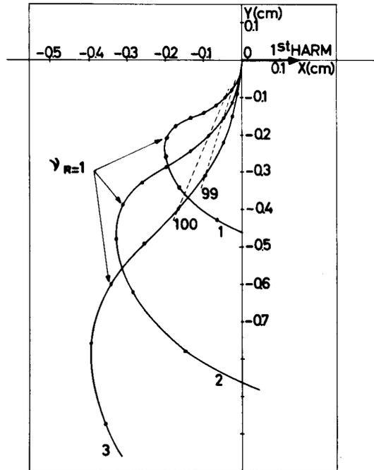
Fig. 2. Motion of the orbit centre for a first harmonic field component only. The dots represent the turn-number. Curve 1:  $A_1$  from 0 to  $0.75 \times 10^{-3}$ , curve 2:  $A_1$  from 0 to  $1.5 \times 10^{-3}$ , curve 3:  $A_1$  from 0 to  $3 \times 10^{-3}$
