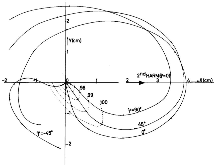
Fig. 3. Motion of the orbit centre for the first and second harmonic components.  $\psi$  is the angle of the first harmonic.  $A_1$  from 0 to  $6 \times 10^{-3}$ ,  $A_2$  from 0 to  $12 \times 10^{-3}$
