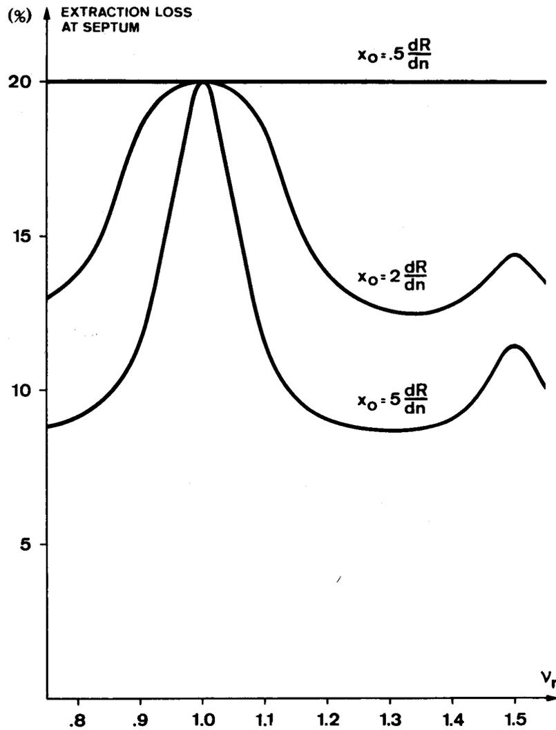
Fig. 7. Monte Carlo calculation of particle loss at septum. Assumptions are: septum thickness  $\delta_{\text{eff}}$ , no losses at side walls of septum nor at the antiseptum, fixed radial gain per turn  $dR/dn = 5 \times \delta_{\text{eff}}$ , uniform energy distribution of particles. The plot shows losses as a function of  $\nu_r$  for different incoherent amplitudes  $x_0$
