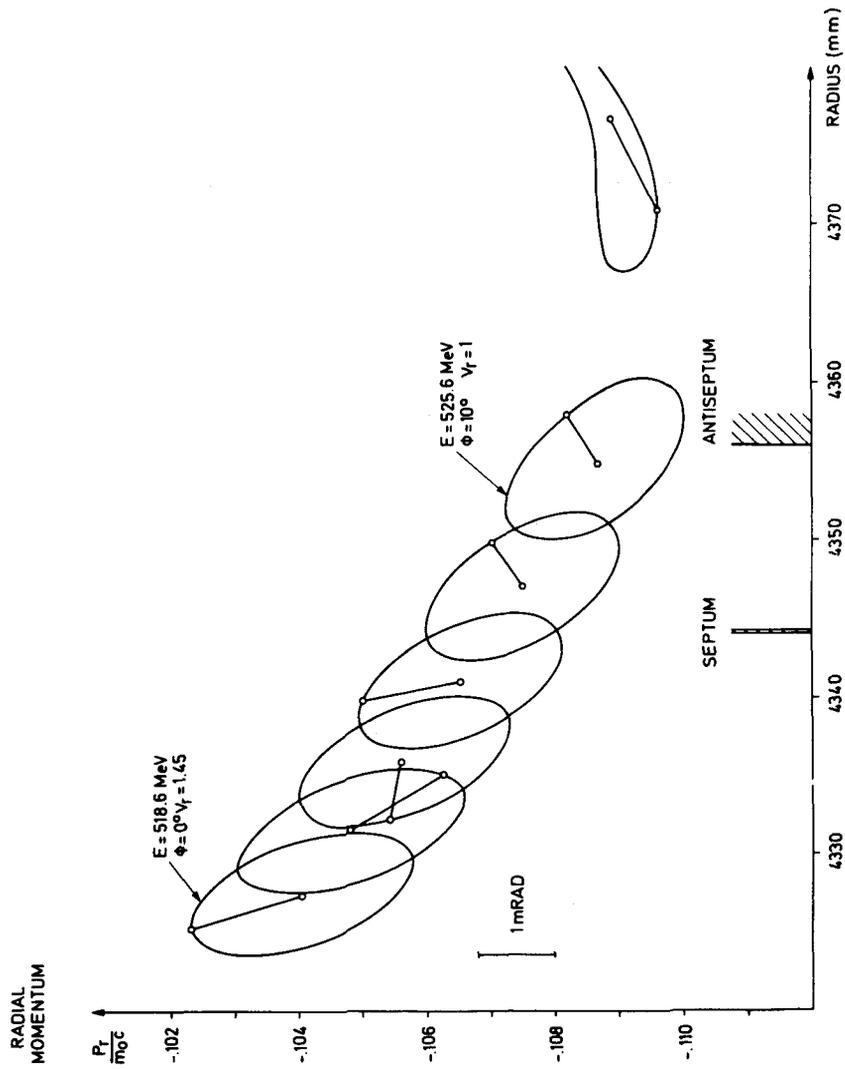
Fig. 2. Radial phase space at septum entrance for SIN ring cyclotron (old design of 52.5 MeV). Assumptions were: conservative beam quality of 50 mm mrad at injection (68 MeV). 400 kV peak voltage on a cavity (1.4 MeV energy gain at extraction, 10° phase slip). Plot shows rapid change of  $v_r$  distorted beam in fringe field and optimum septum position
