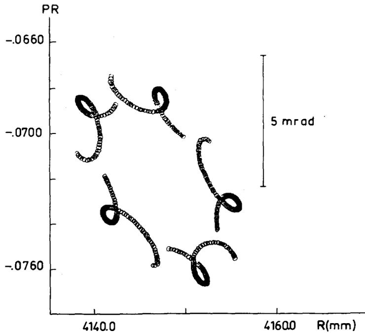
Fig. 9. Coupling resonance  $\nu_r = 2\nu_z$ . The motion of a particle with initial amplitudes of  $x_0 = 9$  mm,  $z_0 = 10$  mm is plotted in phase space every  $45^\circ$  in the 8-sector SIN Cyclotron.  $\nu_r \sim 1.60$ ,  $\nu_z \sim 0.79$ , no acceleration. The curls in the radial diagram indicate the non-linear influence of the vertical amplitude on the radial motion ( $\nu_r$  - shift)
