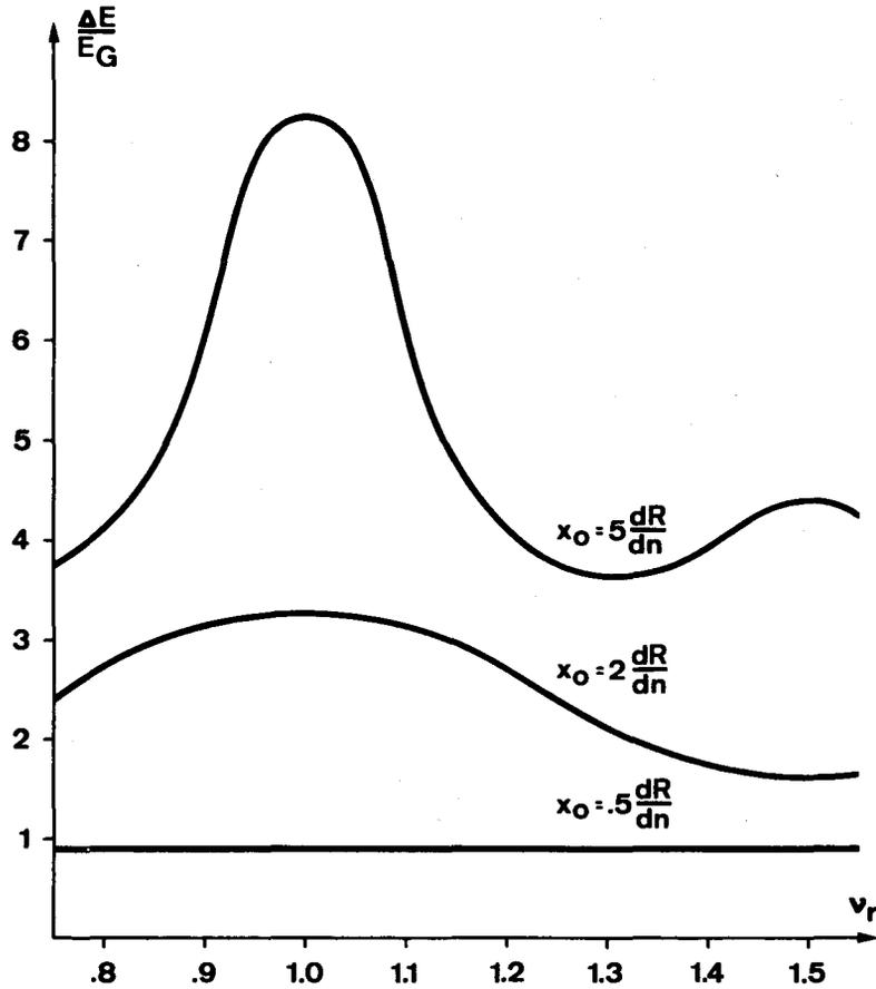
Fig. 8. Monte Carlo calculation of energy spread (FWHM) of extracted beam. The assumptions are the same as for Fig. 7. The plot shows the energy spread  $\Delta E$  divided by the energy gain per turn. The advantage of a good beam quality is obvious
