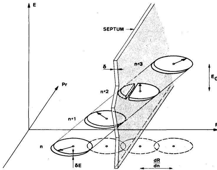
*Fig. 6. Energy distribution of beam at septum entrance. Movement of particles in three-dimensional phase space as a function of turn number  $n$ . In the 'monoenergetic case all particles are inside a thin energy slice  $\delta E$ . In the continuous energy case the distribution is uniform. The plot displays the energy gain per turn  $E_G$ , the radial gain  $dR/dn$ , the projected beam ellipses and the rotation of particles around the centre of the beam ( $\nu_r$ )*
