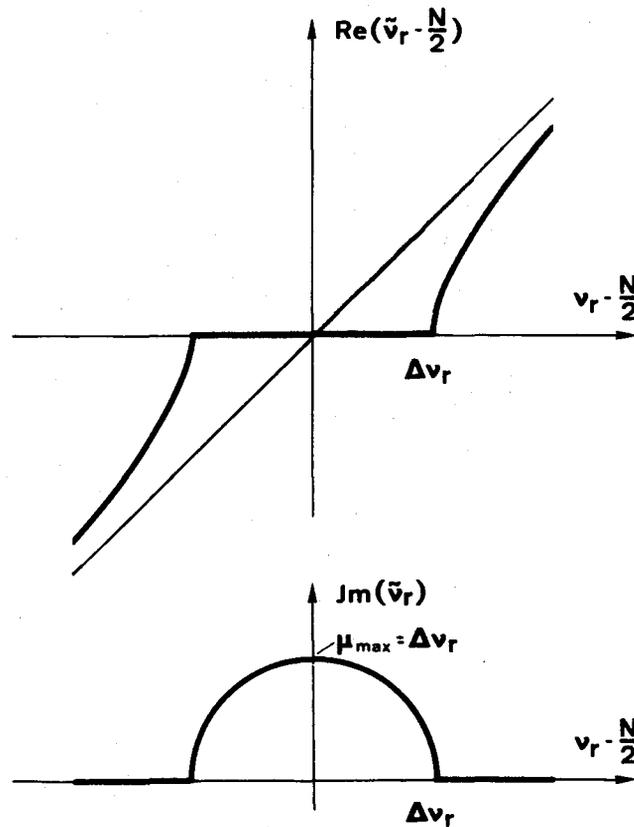
Fig. 4. Stop band  $\nu_r = N/2$ . A gradient bump  $\Delta B(r, \theta) = g_N (r - r_N) \cos N(\theta - \theta_N)$  shifts the betatron frequency  $\nu_r$  to the new value  $\nu_r$ , which is complex inside the stop band. The imaginary part  $Im(\tilde{\nu}_r)$  is responsible for an exponential growth of the radial amplitude
