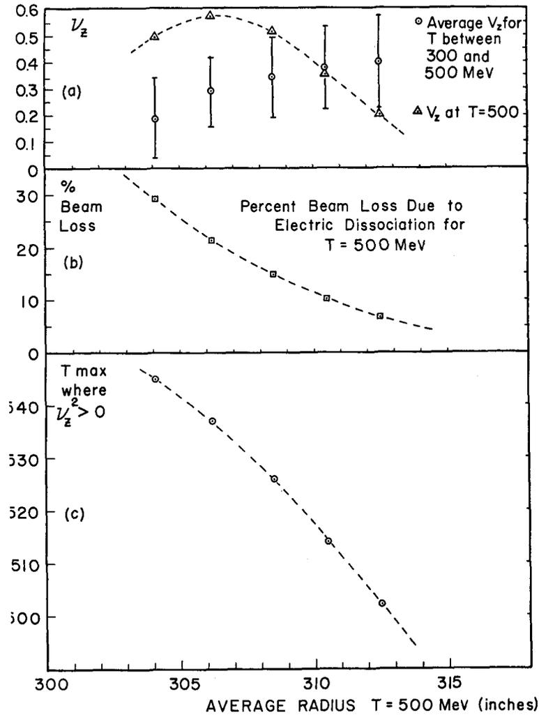
Fig. 4. (a) The variation of  $\nu_z$  with the average radius of the 500 MeV beam;
