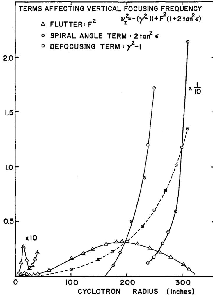
Fig. 1. Terms affecting the vertical focusing frequency  $\nu_z$
