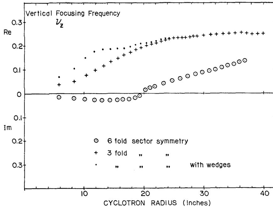
Fig. 6. Changes in  $\nu_z$  due to the changes in the centre region geometry
