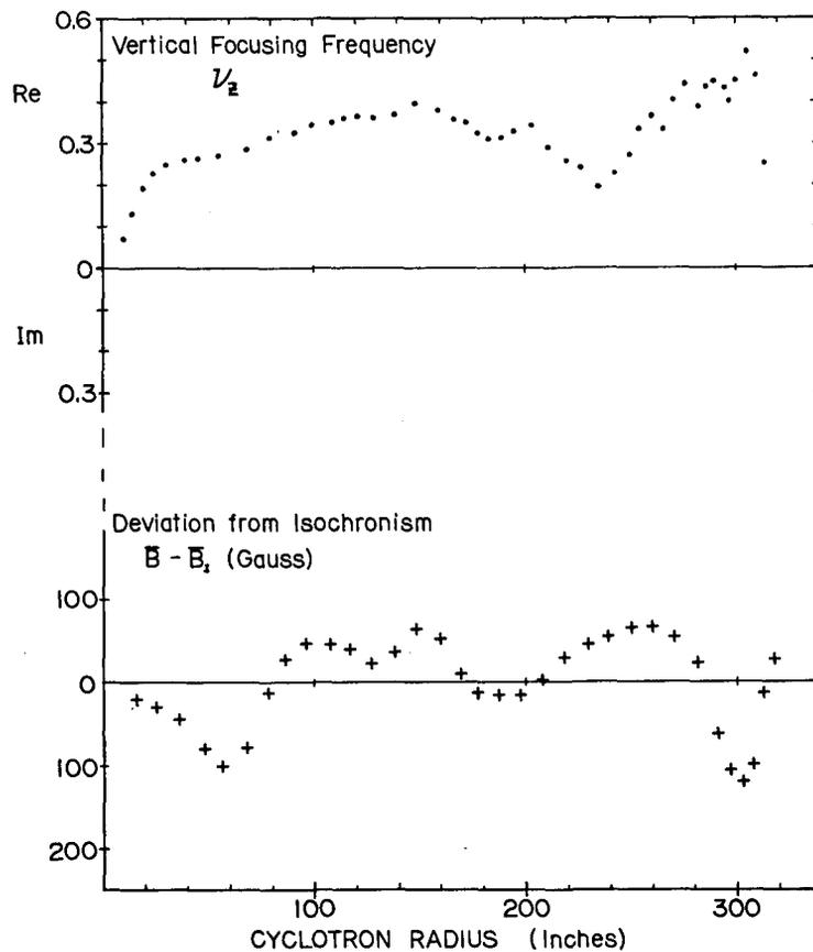
Fig. 3. Properties of tailored magnetic field measured in the models
