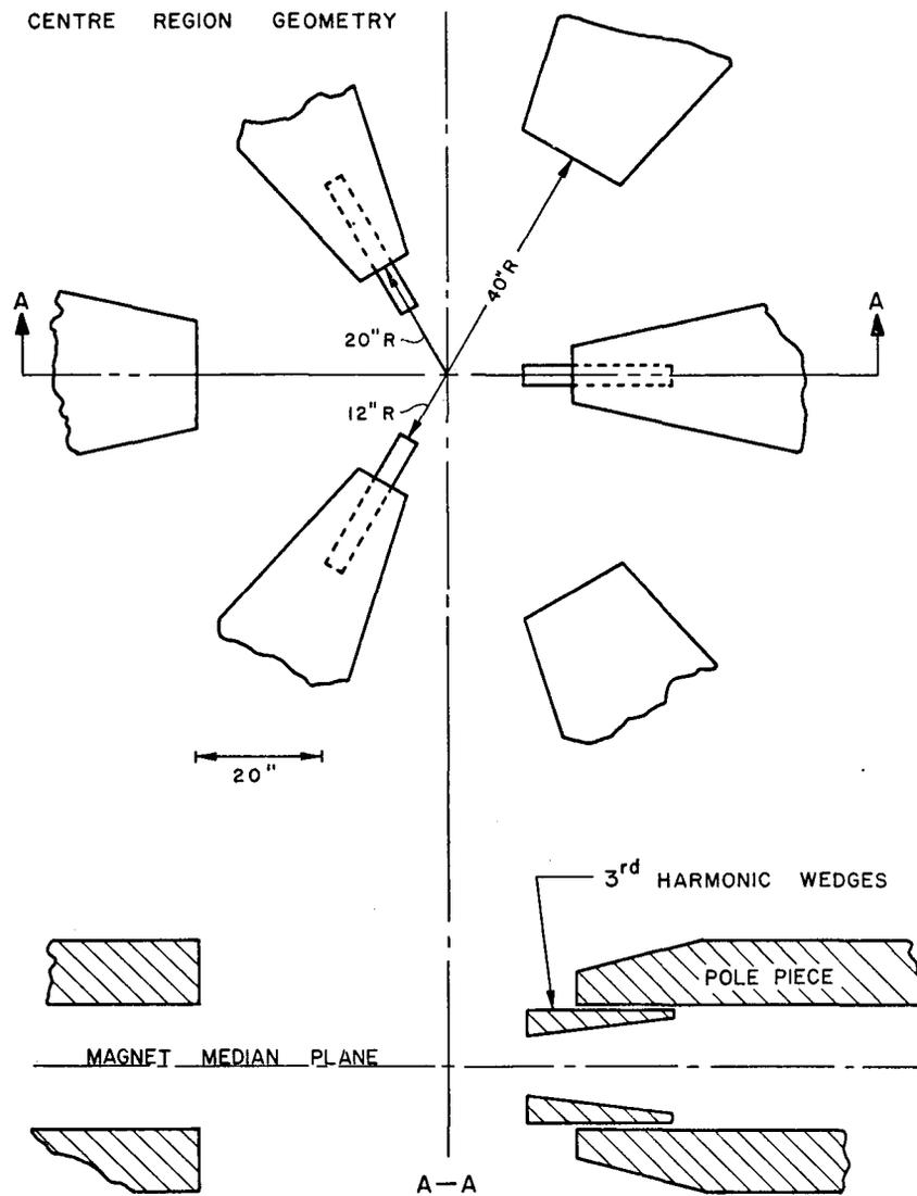
Fig. 5. Details of the magnet centre region showing the cut back sectors and wedges
