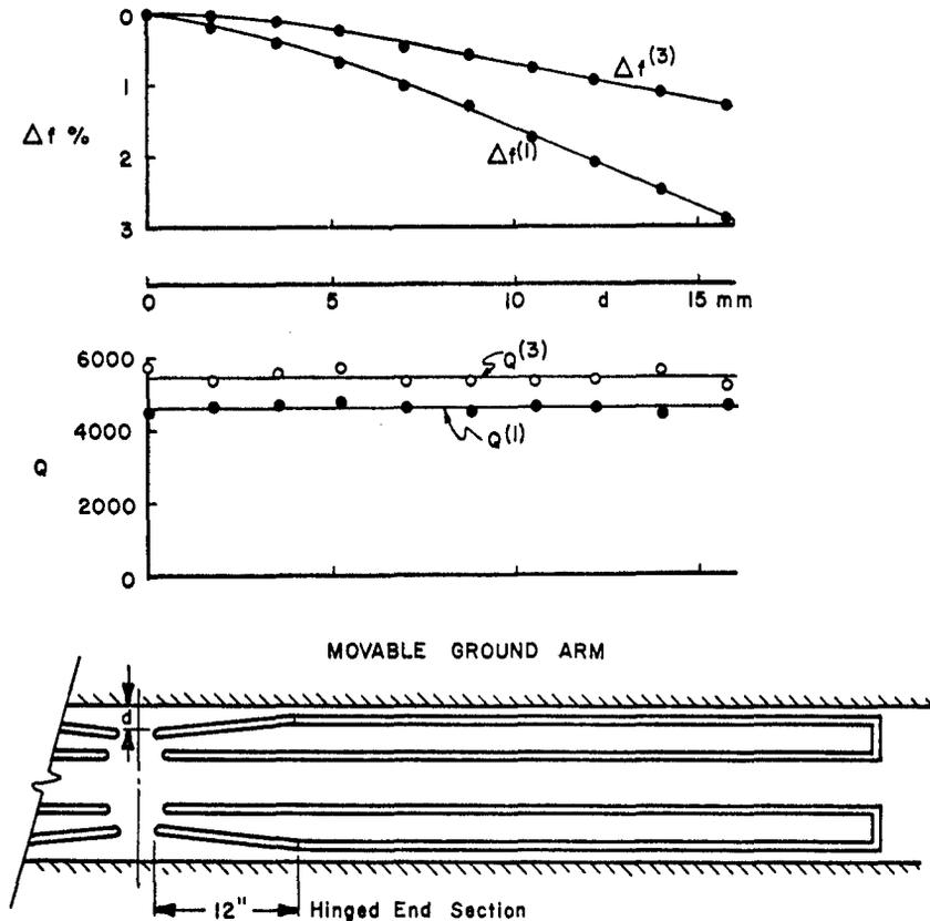
Fig. 3. Variation of the resonant frequency and  $Q$  of the cavity with the motion of capacitor tuning plates at the accelerating gap
