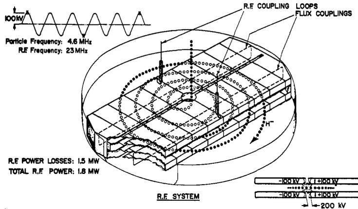
Fig. 1. An isometric view of the resonators and coupling loops in the vacuum tank of the cyclotron
