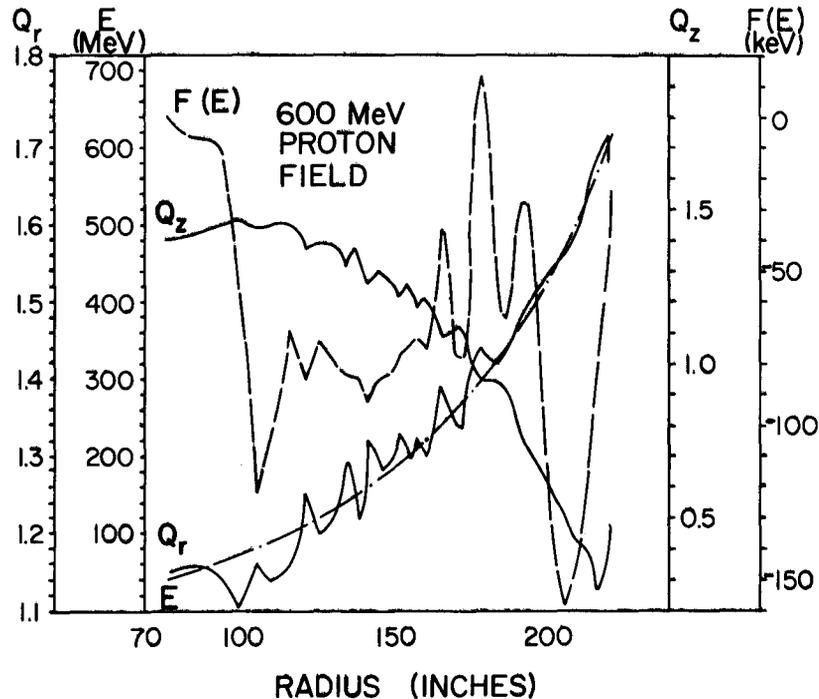
Fig. 3. Graph of energy, radial and axial focusing frequencies and phase slip integral vs radius in the trimmed magnetic field with trim coil currents set for proton operation. With an energy of 600 keV per turn the  $F(E)$  curve gives a phase excursion of  $\pm 22^\circ$
