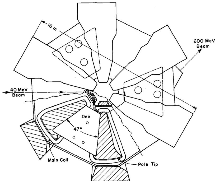
Fig. 2. Plan view of proposed ring cyclotron with central region option 1r
