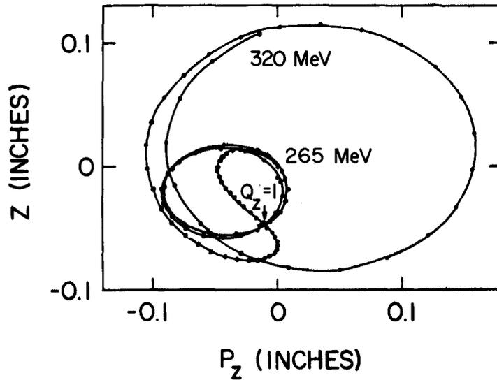
Fig. 5. Repeat of the acceleration run of Fig. 4 but with the median plane correcting coil turned on and roughly optimised. (Note the change in scale relative to Fig. 4)
