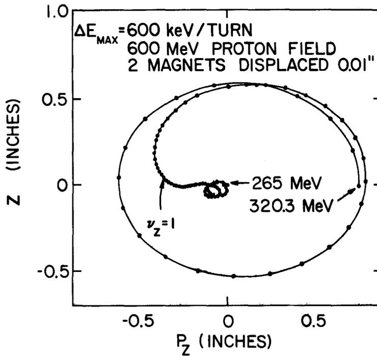
Fig. 4. Plot of  $Z$  vs  $P_z$  on successive revolutions for an orbit accelerated through the  $Q_z = 1$  resonance. Two magnets  $180^\circ$  apart are displaced up and down by  $0.01$  in respectively
