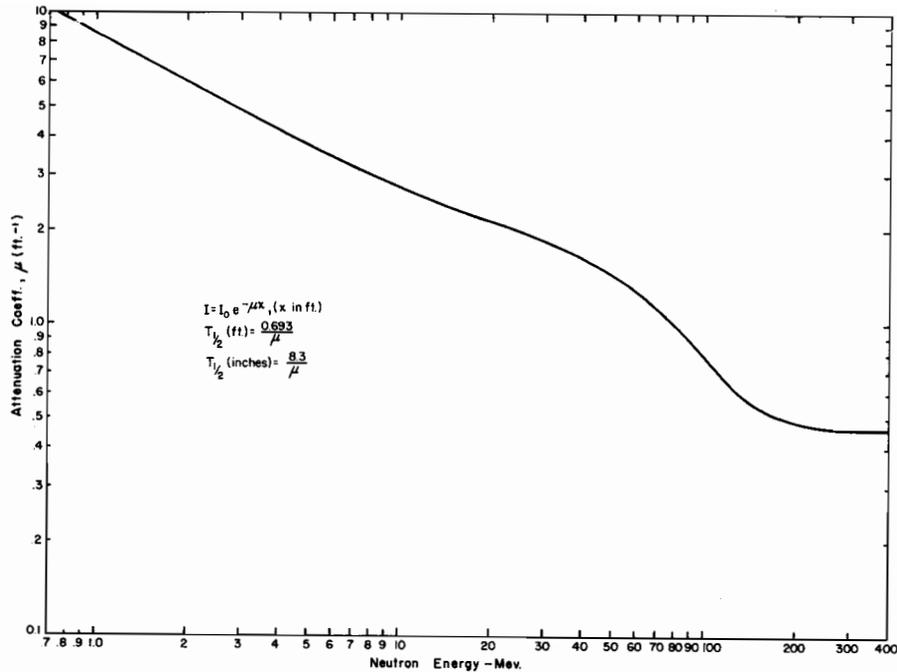
Fig. 250. Attenuation coefficient versus neutron energy for thick shields of ordinary structural concrete ( $2.4 \text{ g/cm}^2$ ).
