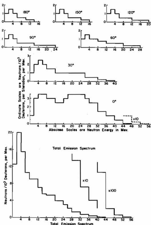
Fig. 249. Neutron spectra in various directions from a thick beryllium target. Also total emission spectrum obtained by compounding the former multiplied by appropriate solid angle factors. Deuteron energy 60 Mev.
