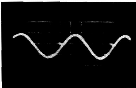
Fig. 207. Beam signal superposed on r-f signal.
