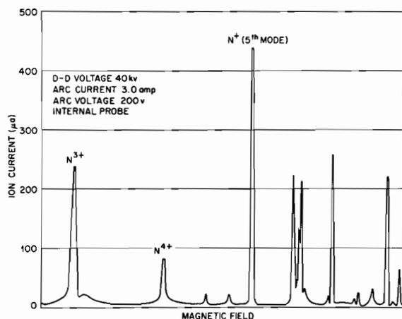
Fig. 209. Magnetic analysis of ion current in ORNL 63-inch cyclotron, at full radius.
