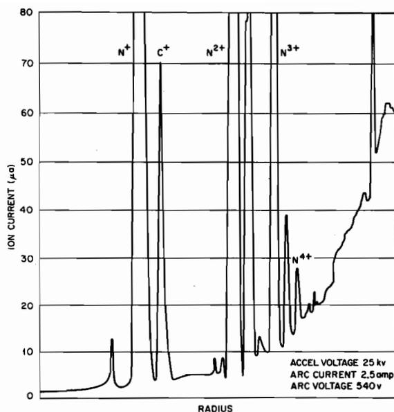
Fig. 210. Ion spectrum obtained at 180° in D-C test of source for heavy ions.
