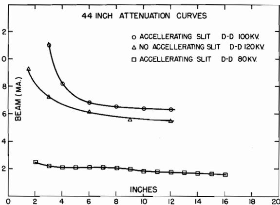
Fig. 204. Beam attenuation in ORNL 44-inch cyclotron.
