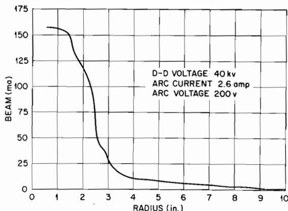
Fig. 206. Attenuation of beam from grid-type ion source.
