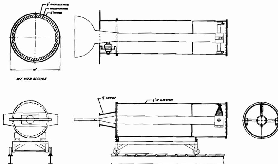
Fig. 162. The dee, dee stem, and dee-stem tank, shown rolled back from the cyclotron. Not shown is the r-f power amplifier which will be mounted on the side of the tank.
