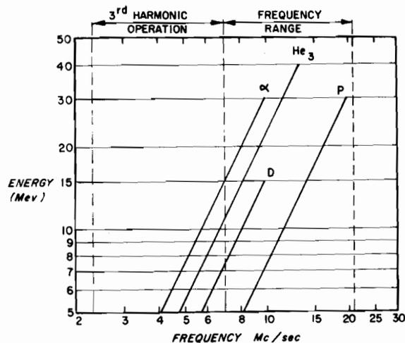
PARTICLE ENERGY AS A FUNCTION OF RADIO FREQUENCY FOR AN EXTRACTION RADIUS OF 60 cm. THE MAXIMUM ENERGY CORRESPONDS TO A CENTRAL MAGNETIC FIELD OF 13 KILOGAUSS.
