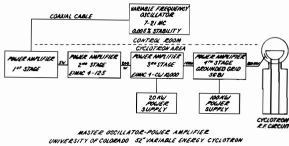
Fig. 163. Block diagram of the r-f system.
