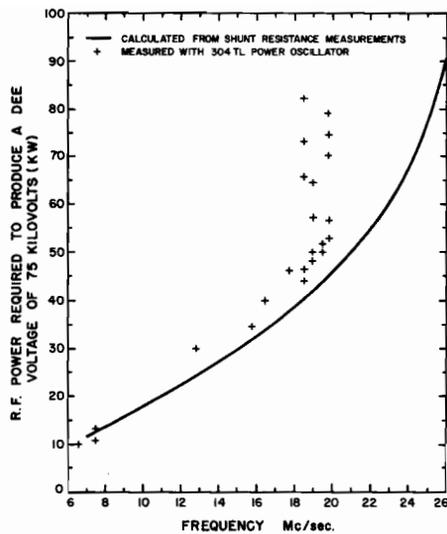
Fig. 165. Experimental results obtained with the full-scale model of the resonant circuit model.
