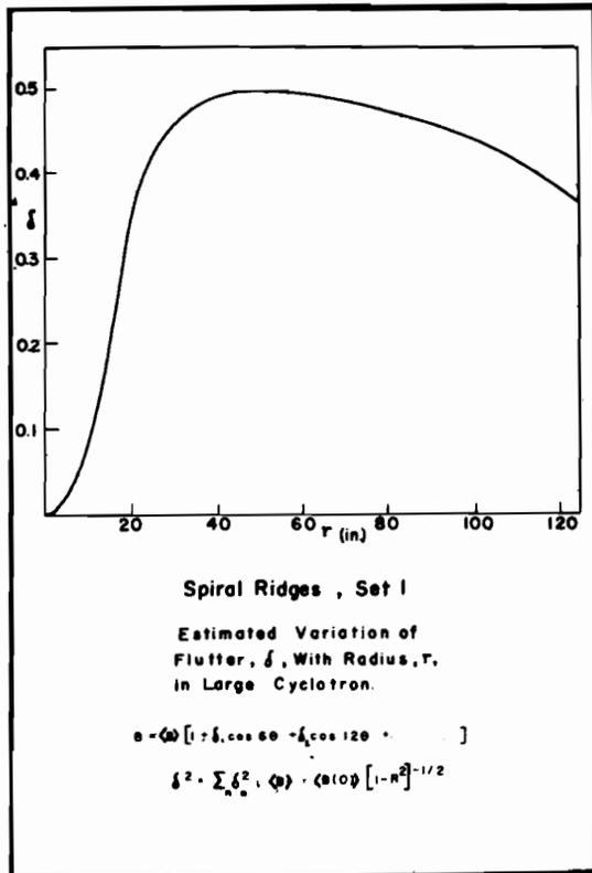
Fig. 19. Estimated flutter vs radius
