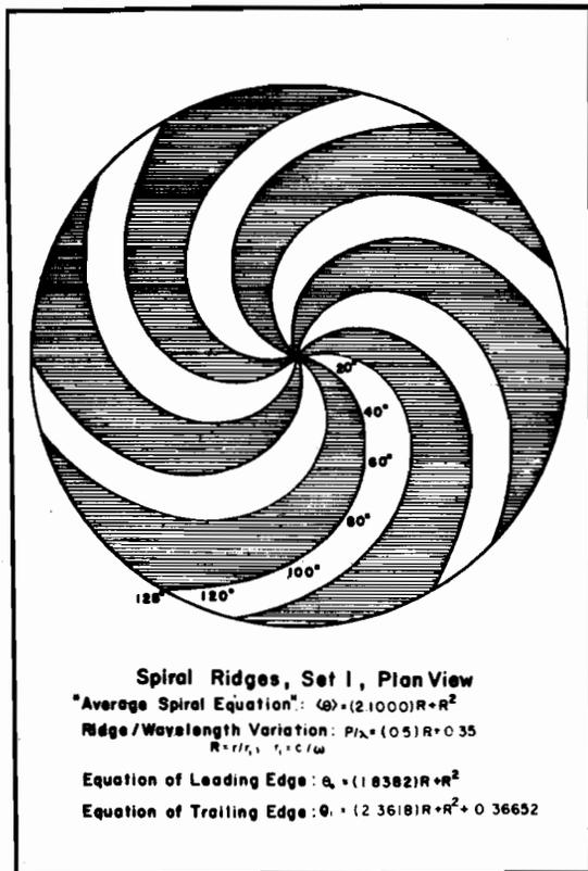
Fig. 17. Plan view of "low-field" poleface
