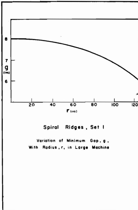
Fig. 18. Variations in minimum gap with radius
