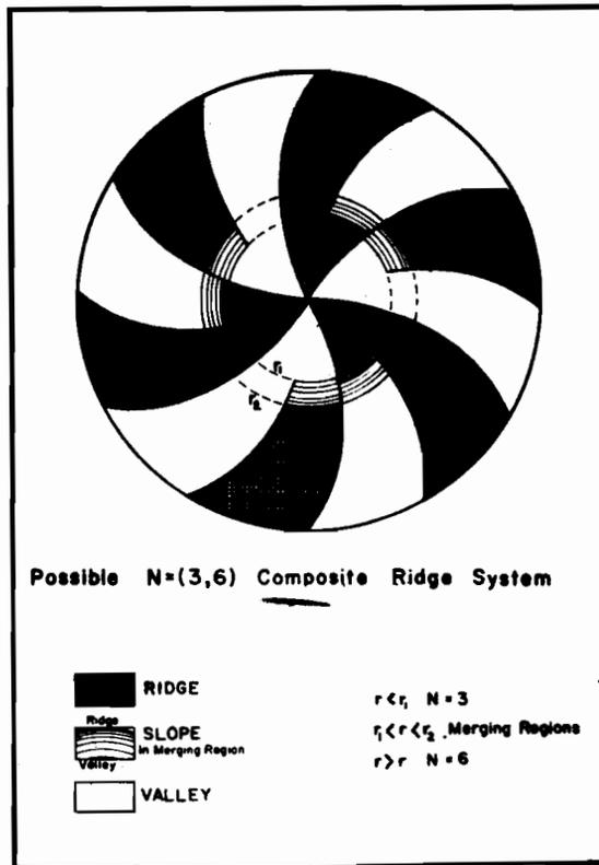
Fig. 20. Composite, (N=3-6) "high-field" design
