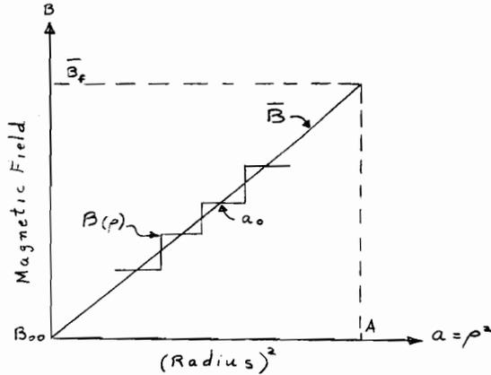
Fig. 4. Approximating the isochronous magnetic field by the use of a number of circular trimming coils.
