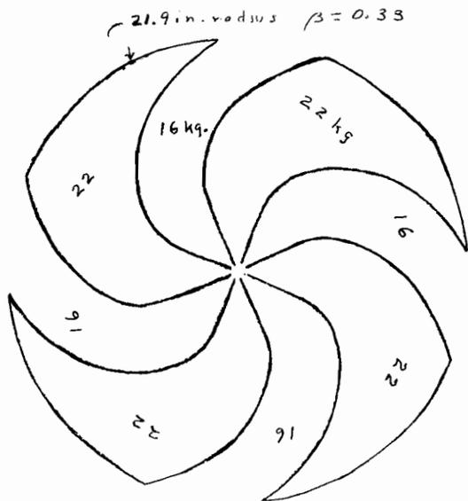
Fig. 2. A magnetic field geometry employing constant hill and valley fields.
