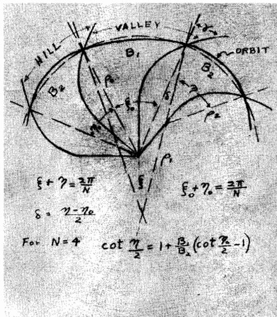
Fig. 1. The solid curve represents part of the ion orbit compared with a circle.
