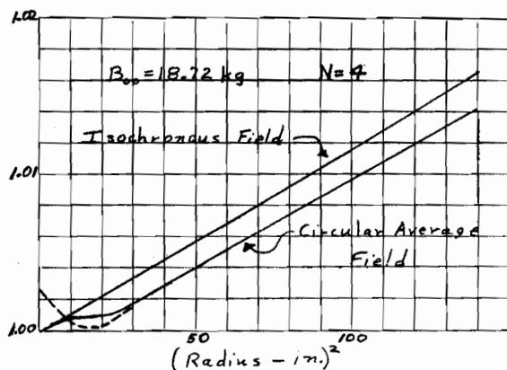
Fig. 5. The isochronous field near the center of the UCLA cyclotron and the required circular average field to produce isochronism.
