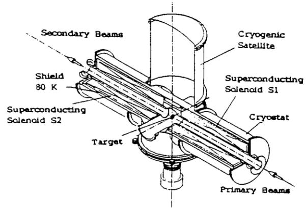
Figure 8 : Schematic view of the cryostat of SISSI.
