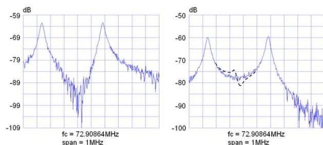
Figure 3: Pickup coupling measured with network analyzer at an inductively coupled dee (left) and at a capacitively coupled dee (right, dashed line showing qualitatively a curve for the 2<sup>nd</sup> mode).
