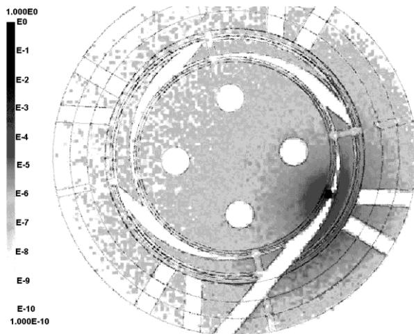
Figure 5: Power density of neutrons produced by a 250 MeV proton beam stopped inside the cyclotron; logarithmic gray scale ranges from  $10^{-10}$  to  $10^0$  W/cm<sup>3</sup>.
