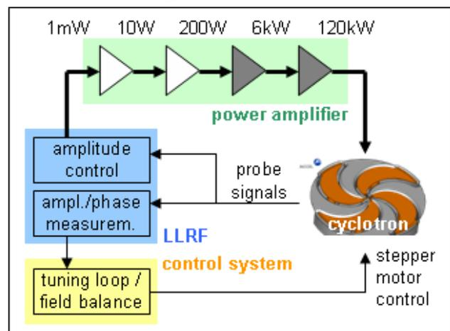
Figure 1: Main components overview of the RF system.
