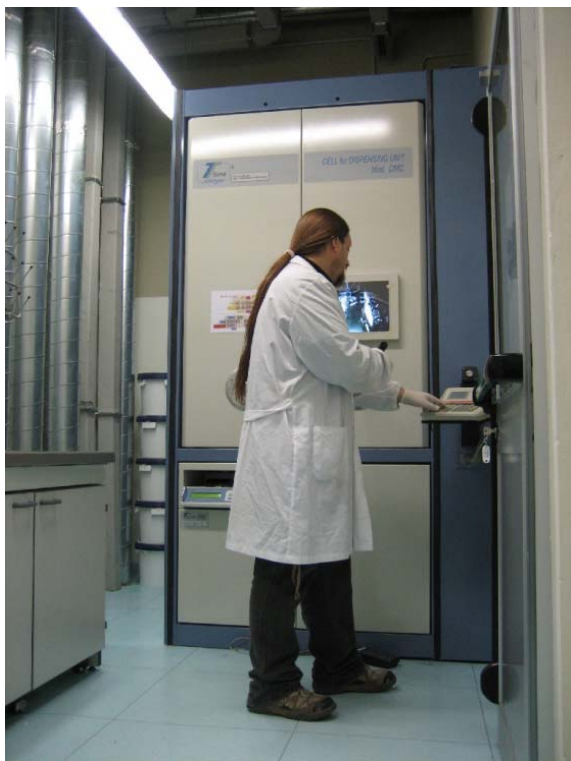
Figure 3: Cell for dispensing unit: an operator during the manipulation of ^{18}\text{F} before the activity measurement
